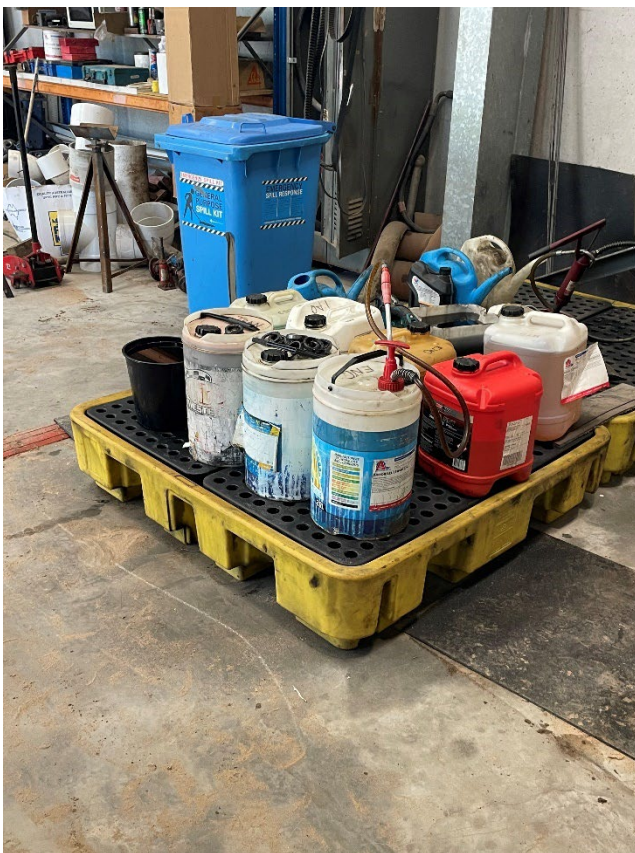
Bunded pallet for fuel storage
