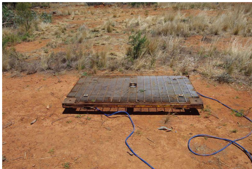
Photo 3. Weighing platform with loads cells located under platform.
