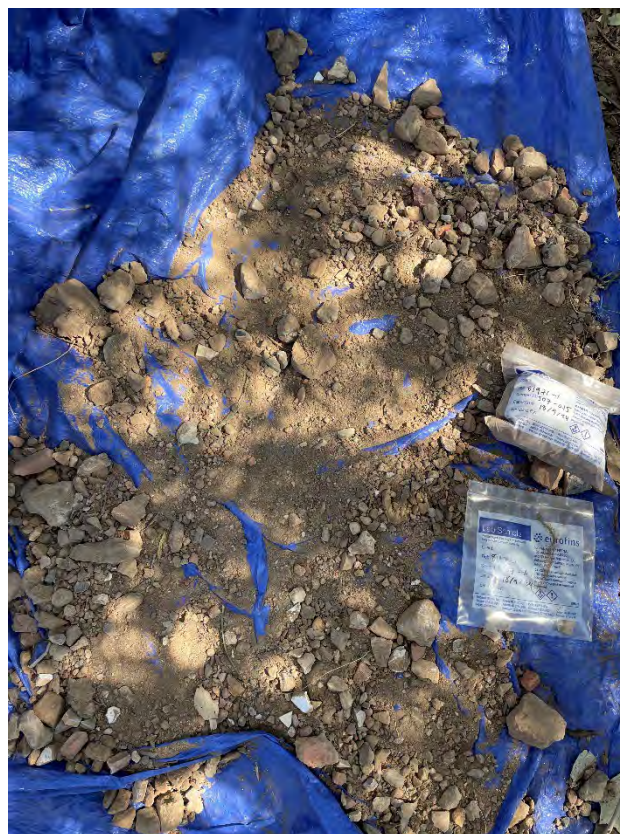
Image 2: Fill Material from Unsealed Driveway located in the south-eastern portion of the site (location of surface soil sample S07 and identified ACM).
