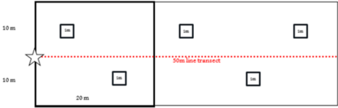
Figure 2.1 Schematic diagram illustrating the layout of the nested 20 x 50m, 20 x 20m and 1 x 1m sub-quadrants used for the assessment of condition attributes at each site
