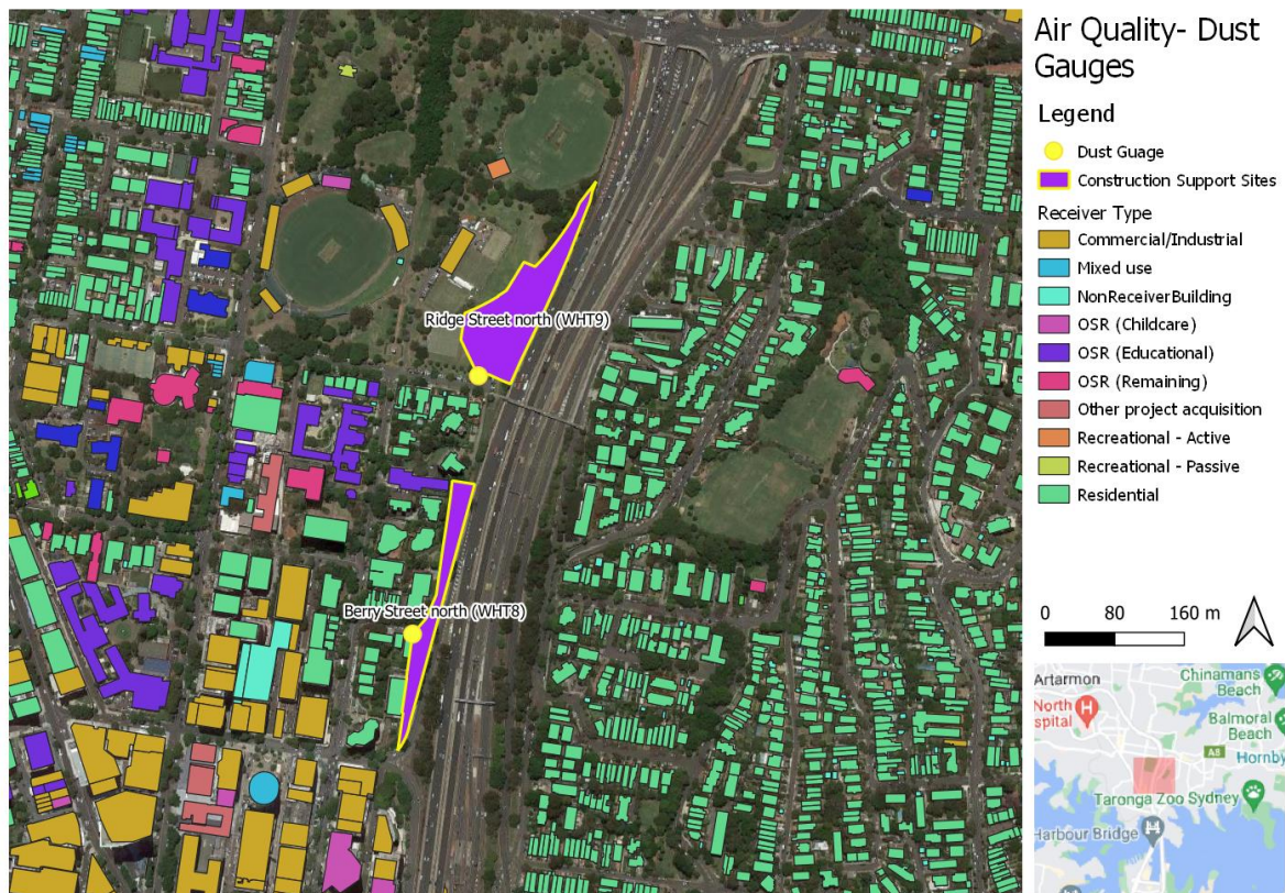
Figure 3-1 Depositional Dust Gauge indicative locations for Ridge Street and Berry Street north
