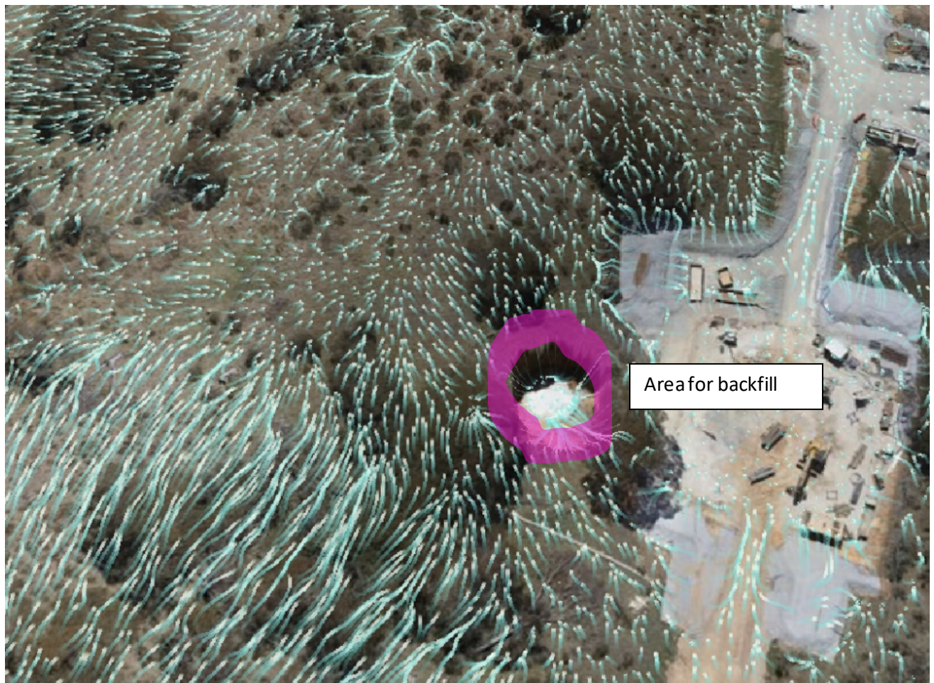
Figure 6: Local surface water flow path and area to be backfilled
