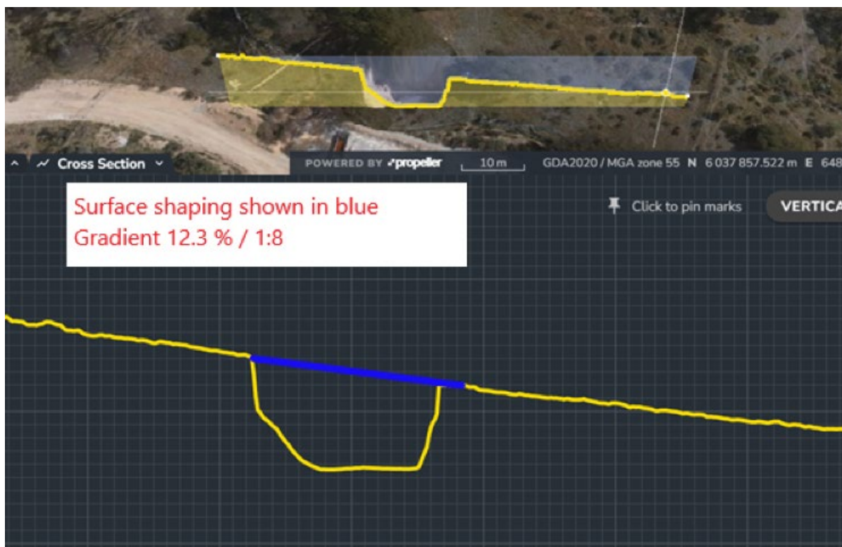
Figure 7: Final landform cross section
