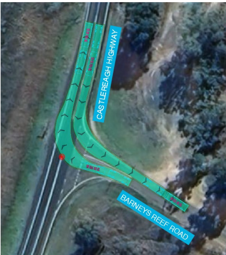
Plate 3.2 Swept path of a 19 m truck and dog trailer at the Castlereagh Highway/Barneys Reef Road intersection
