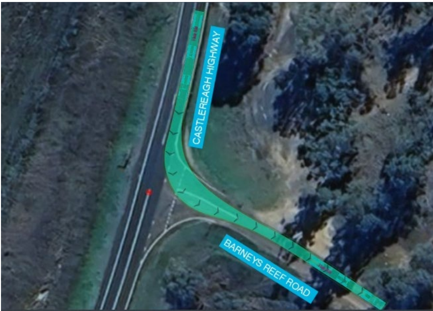
Plate 3.1 Swept path of a B-double at the Castlereagh Highway/Barneys Reef Road intersection
