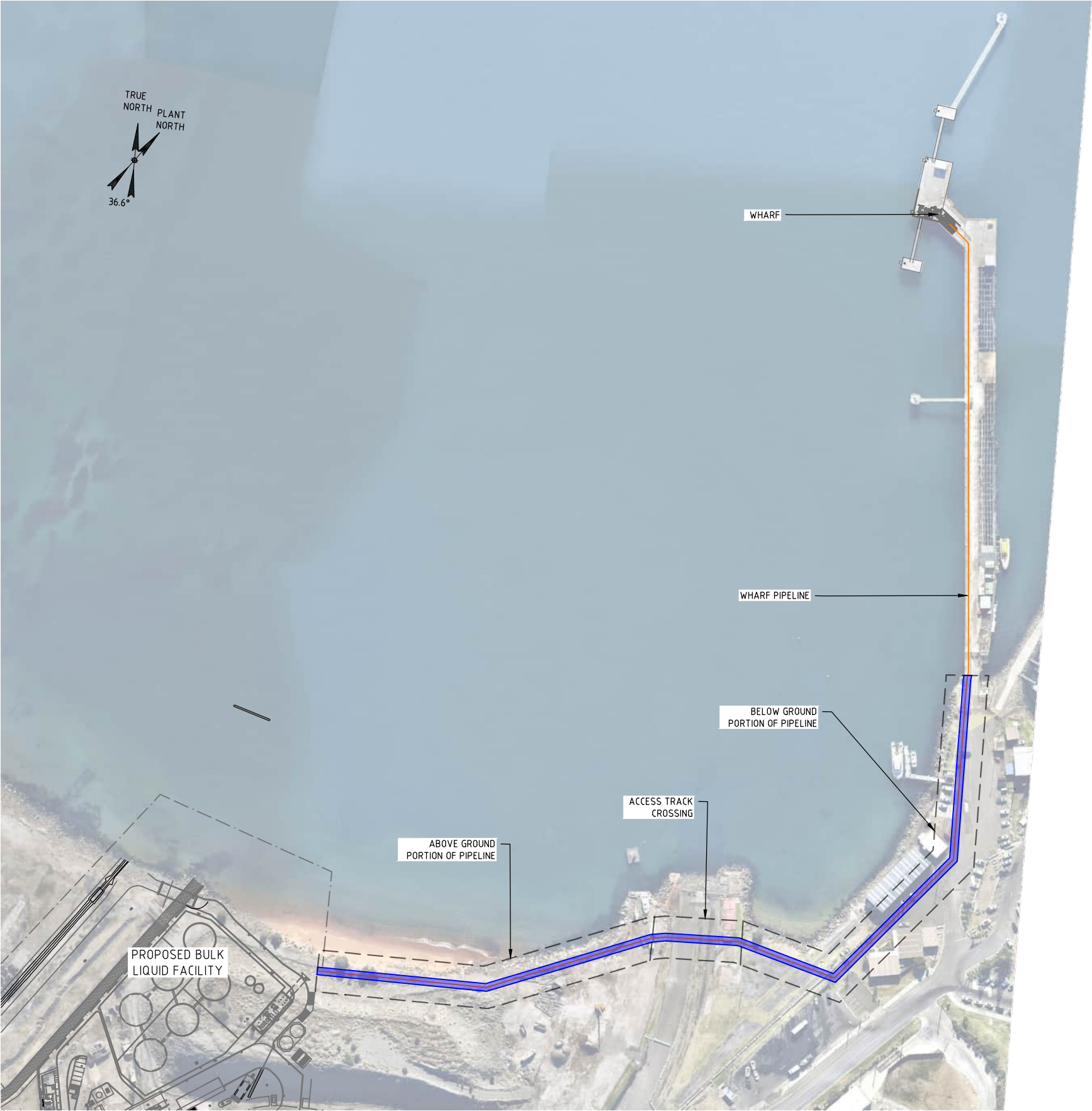
WHARF PIPELINE PLAN 1:2,500
