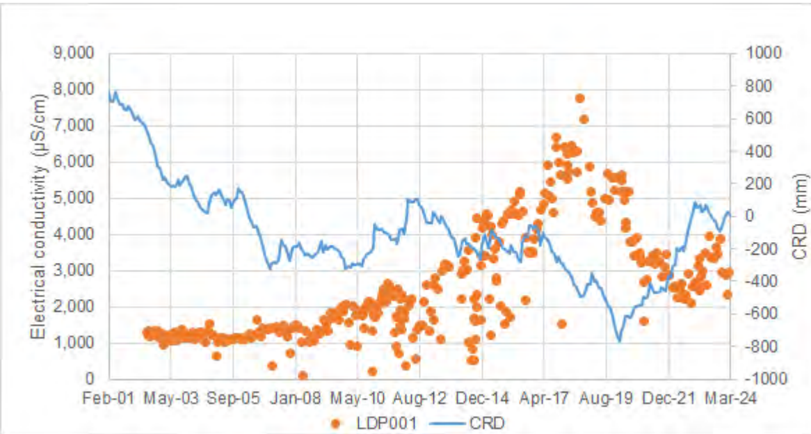
Figure 5-2 Recorded LDP001 discharge electrical conductivity
