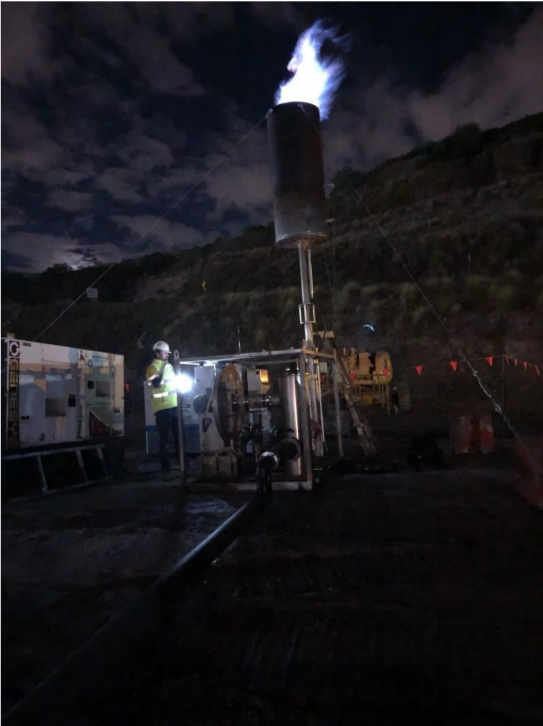
Figure 4: Landfill gas no.1 flare installation at EC REP for pumping trial purposes
