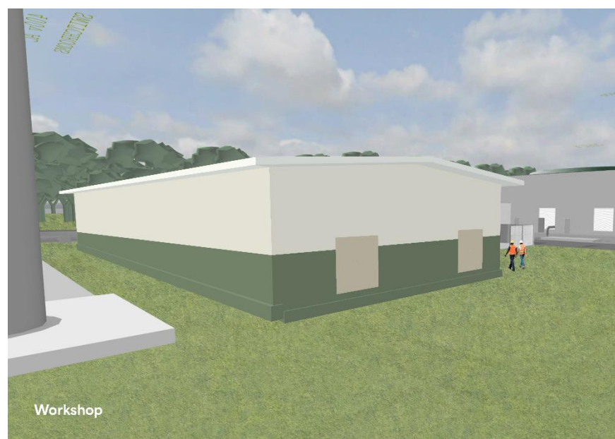
Figure 99 Preliminary design studies for cladding on the Workshop building to reduce solar absorptive criteria.
