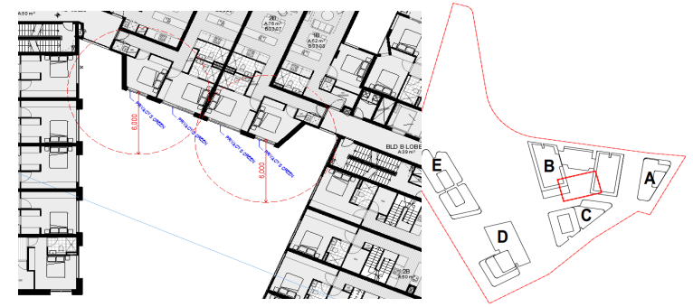
Fig. 3F1.4 Building B Plan. Privacy screens annotated in blue & Key Plan
