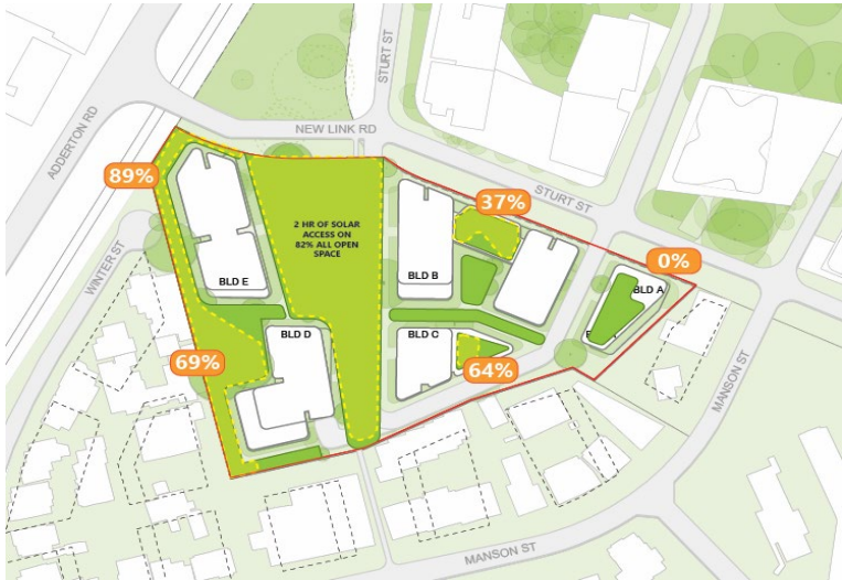
Fig. 3D1.2 Solar Access within Open Space Retention of trees is the main driver for communal open space on ground - as such deep soil areas and communal open space are largely co-located. This along with podium communal spaces creates pocket spaces across the overall development ensures easy access for all users. The variety of open spaces creates easily identifiable spaces for relief.
