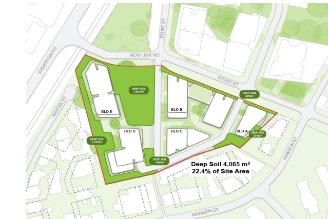
Fig.3E1.1 Deep Soil Diagram The Public open space is intended to support large scale planting, providing for a deep soil zone within the site.
