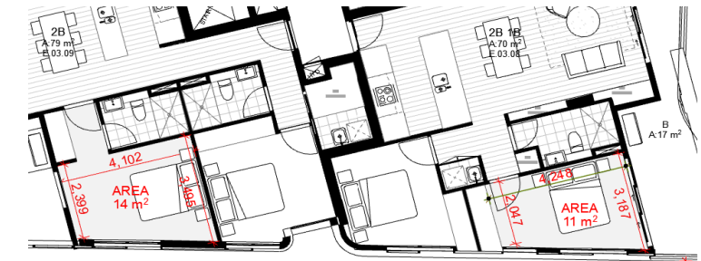
FIG.4D3.1 Example of an irregular bedroom on the south facade where dimensions average to 3m but functional area exceeds the requirement
