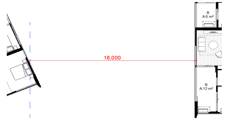
Fig. 3F1.5 Building B separation (storeys 5-8) with blade wall projection to address visual privacy.
