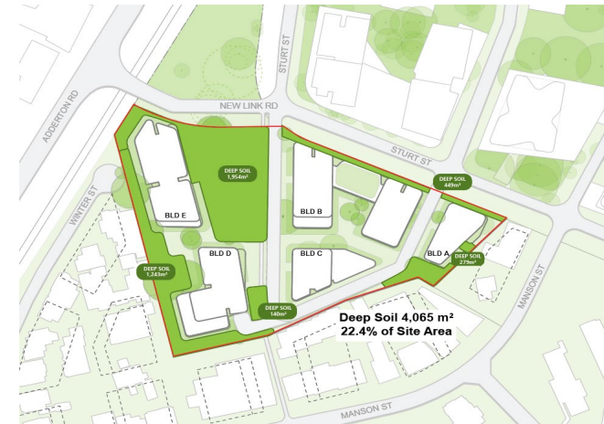
Fig.3E1.1 Deep Soil Diagram The Public open space is intended to support large scale planting, providing for a deep soil zone within the site.
