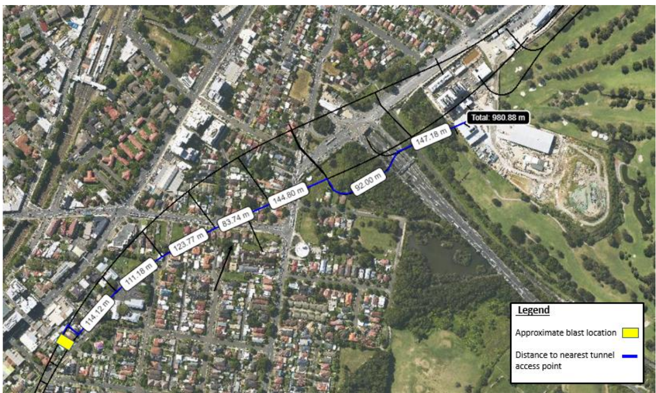
Figure 2 Indicative distance from blasting area to Shed B
