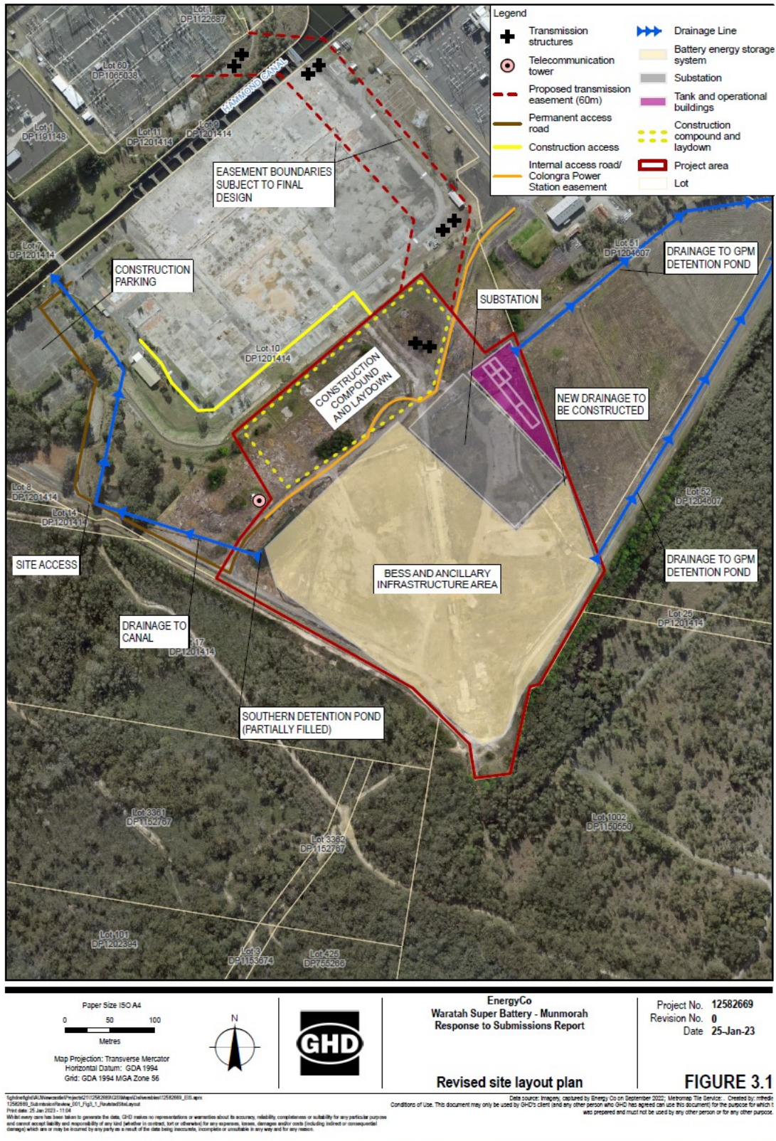
Figure 3 General Construction Arrangement
