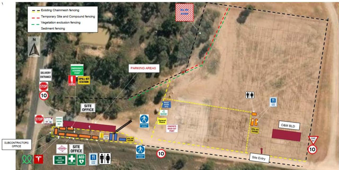
Figure 3: Lot 1 DP1249830 and Lot 2DP1249830 - Stage 2a and Stage 2b (excluding Stage 2b(ii)) Detailed Map - BESS Project site including Construction Compound Area
