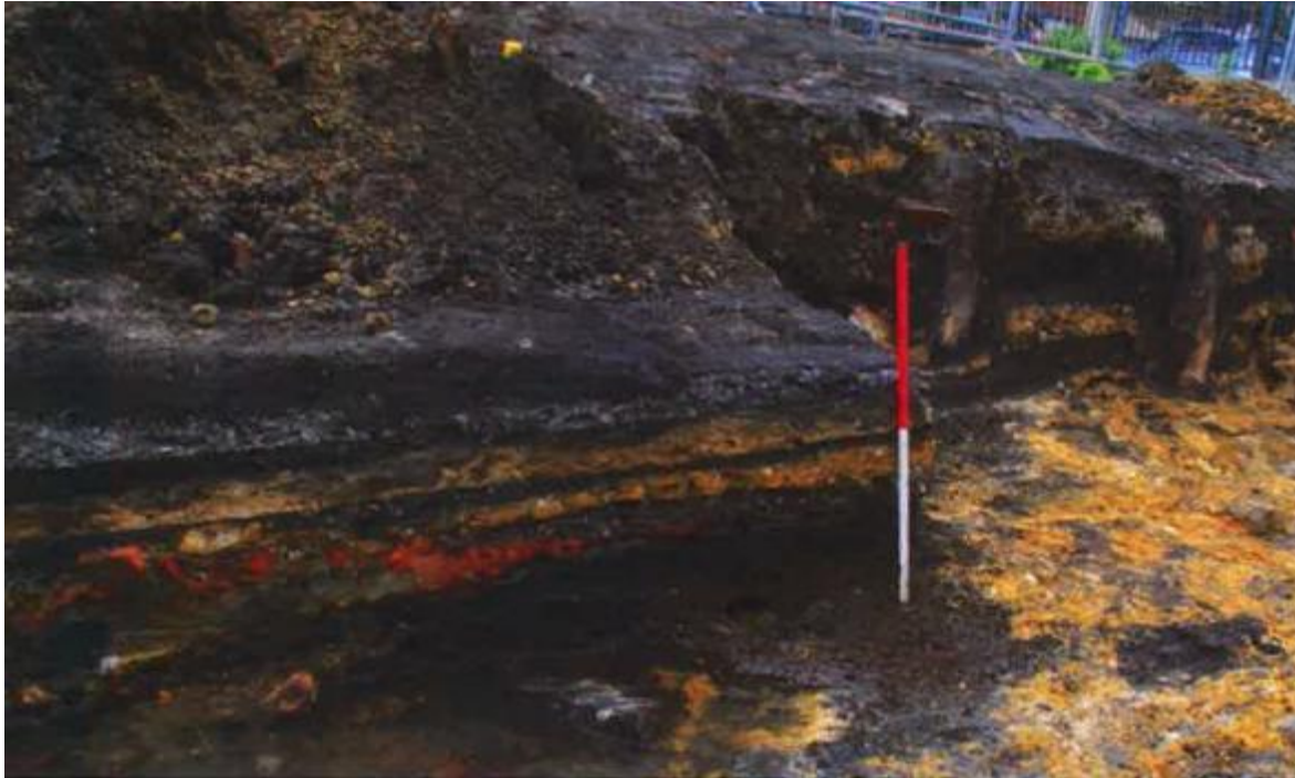
Figure 8: Bulk fill layers identified by Casey & Lowe 2012. Characteristic yellow crushed sandstone is evident 49
