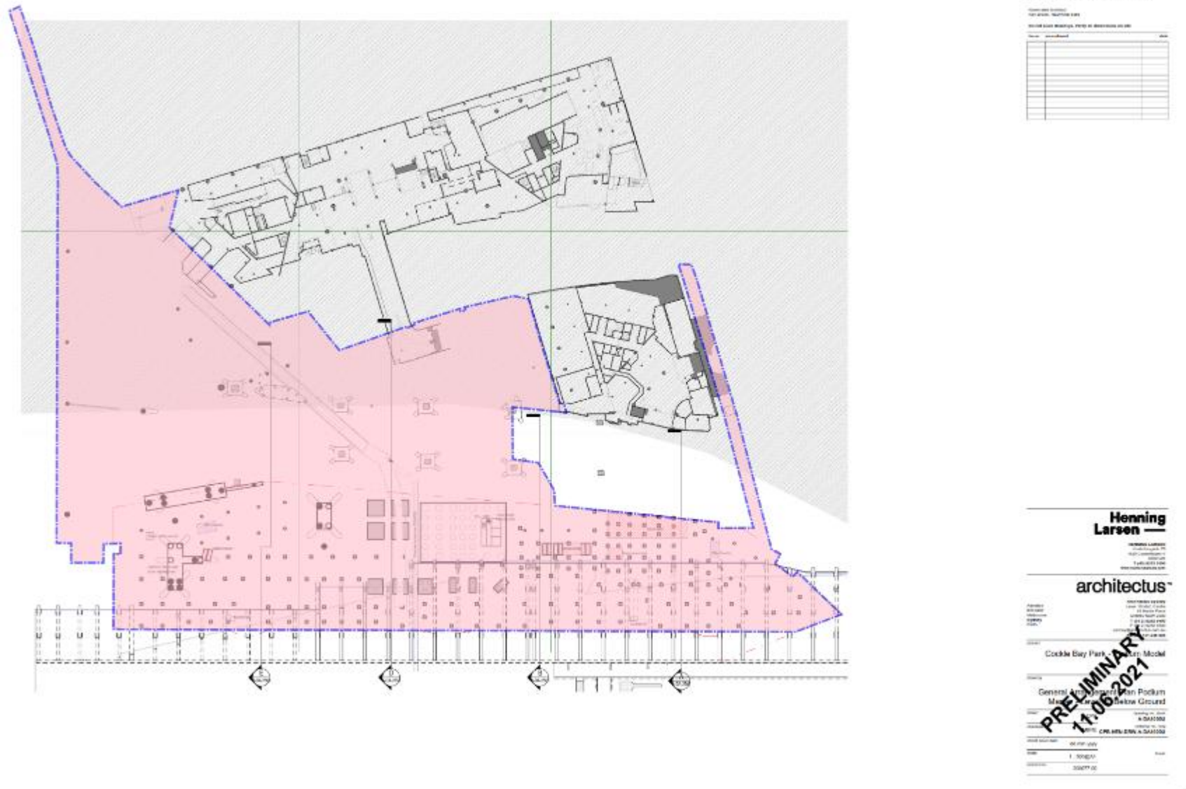
Figure 43: Proposed piling, footing and subsurface utility locations
