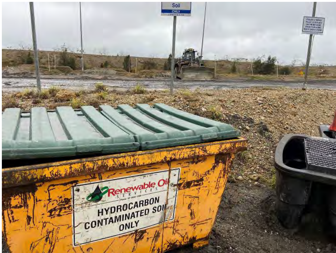
Plate 17 – Minor volume hydrocarbon contaminated waste bin observed to not be watertight.
