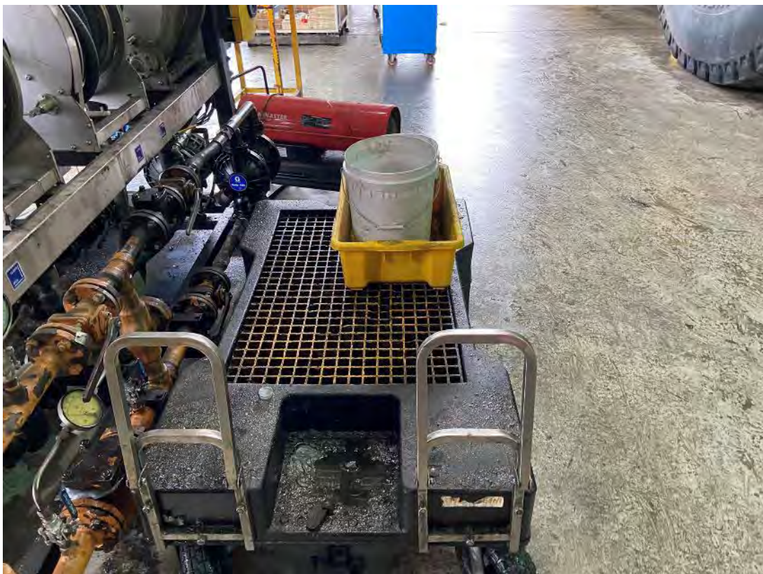
Plate 14 – Mobile bunded trollies utilised in workshop area
