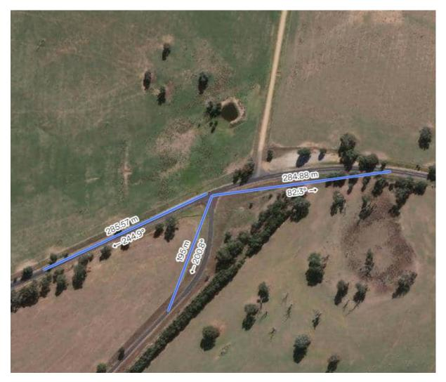
Sight distance is restricted on all approaches. However, mitigation measures have been implemented using intersection warning signs on all approaches. Further this intersection was being upgraded as part of works along Galong Road undertaken in 2022.
