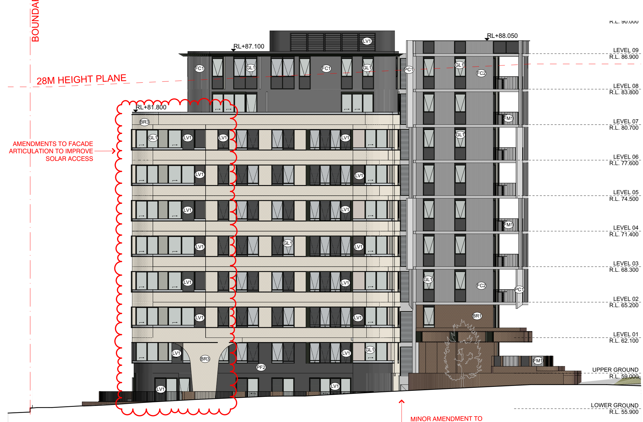
DS - BLDG. D SOUTH ELEVATION SCALE: 1:200@A1
