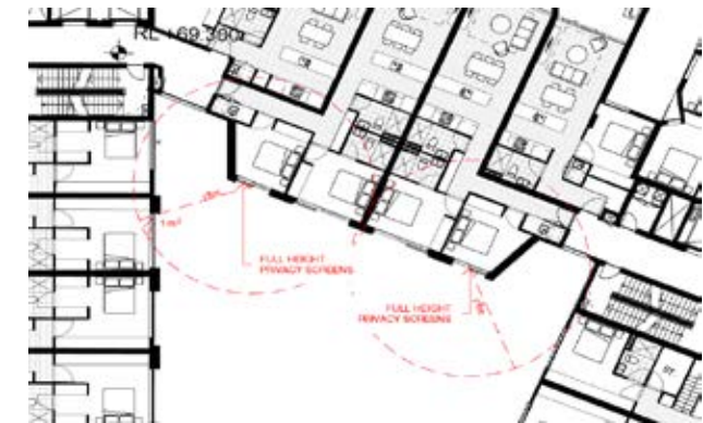
Fig. 3F1.5 Building B non-compliant separation (LUG-L04) & Key Plan
