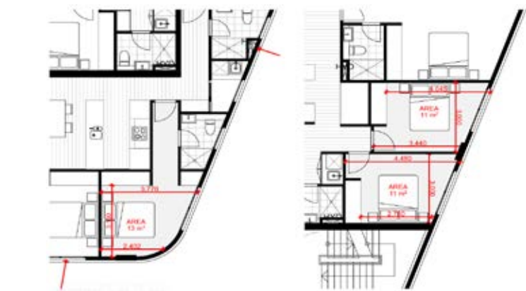
Fig.4D3.1 Example of irregularity. BLD A typical bedroom measurement, functionality of the rooms are maintained.
