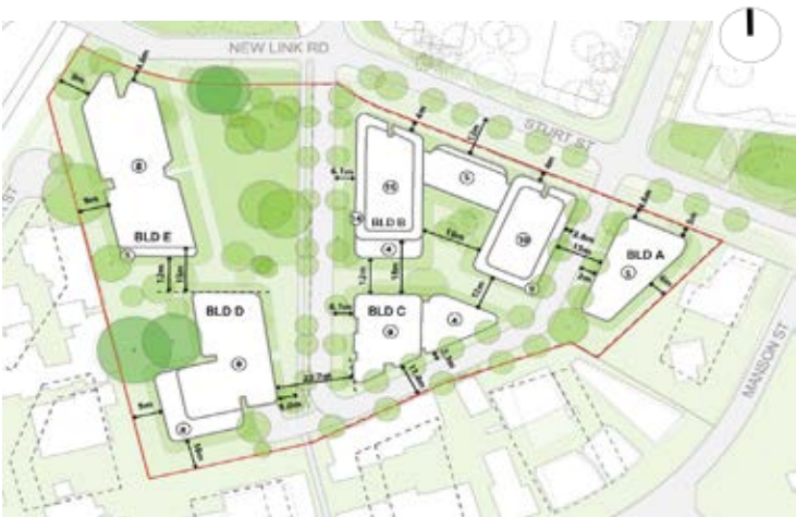
Fig. 3F1.1 Stage 1A Separation Diagram Building Separation on Site (Minor non-compliances)
