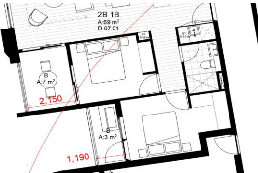
Fig.4E1.2 D.UG.01 - D.08.01 balcony non-compliance
