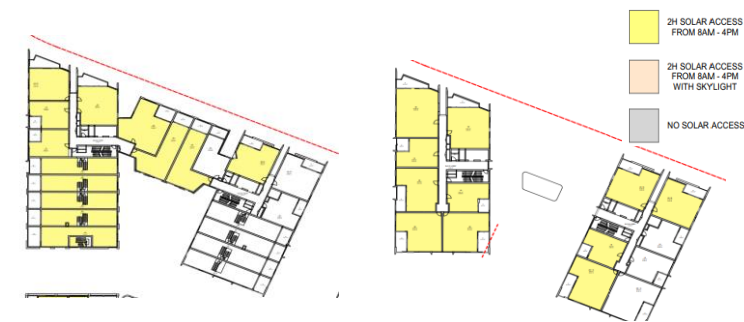
Fig.4A1.1 Solar Amenity Diagram 8am-4pm typical podium (left) and typical tower (right).
