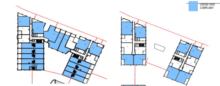
Fig.4A3.1 Cross Ventilation Diagram typical podium (left) and tower (right).
