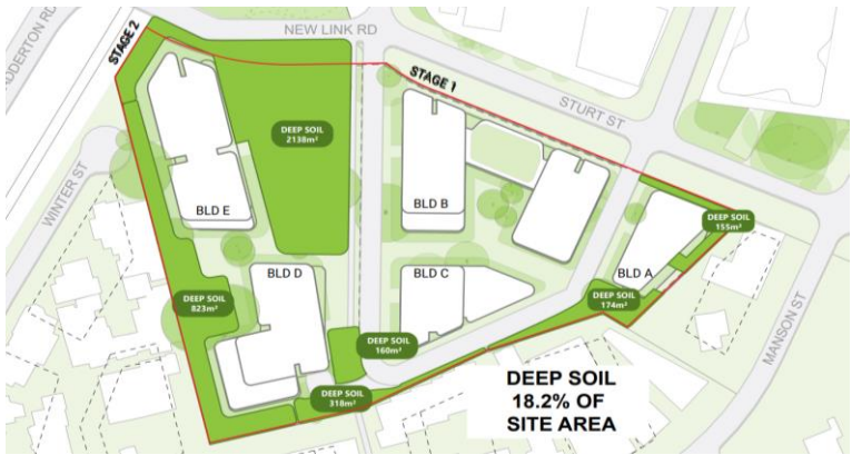
Fig.3E1.1 Deep Soil Diagram The Public open space is intended to support large scale planting, providing for a deep soil zone within the site.
