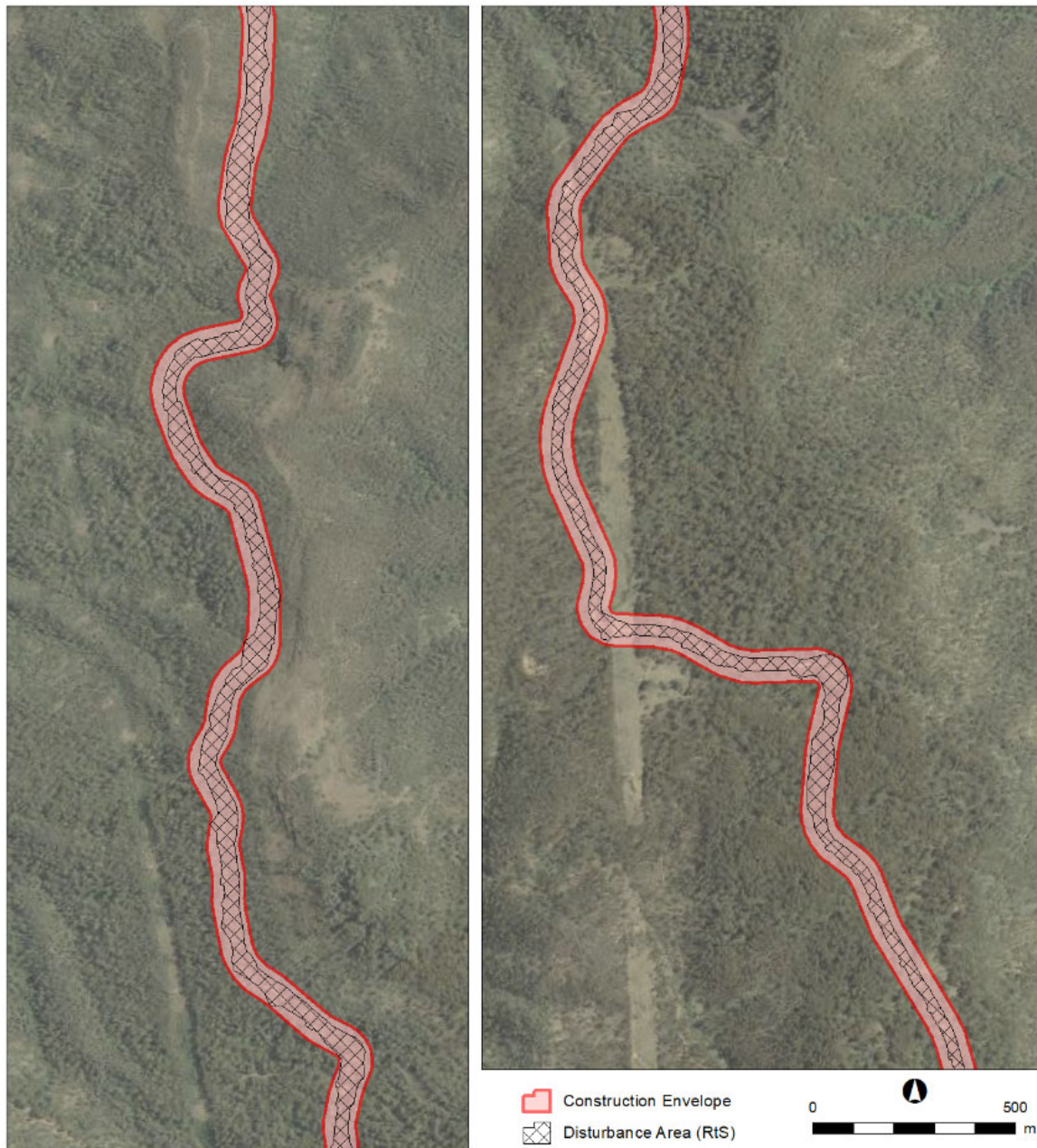
Figure 1-3: Disturbance area and construction envelope
