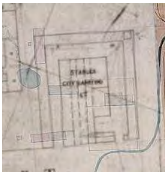
Figure 3.14 Detail of the south eastern corner of the overlay of the 1865 Trigonometrical Survey and 1886 Sydney Water within the footprint of the City Carrying Co. stables. Note the construction materials are indicated: timber (grey), stone (yellow) and brick (pink).
