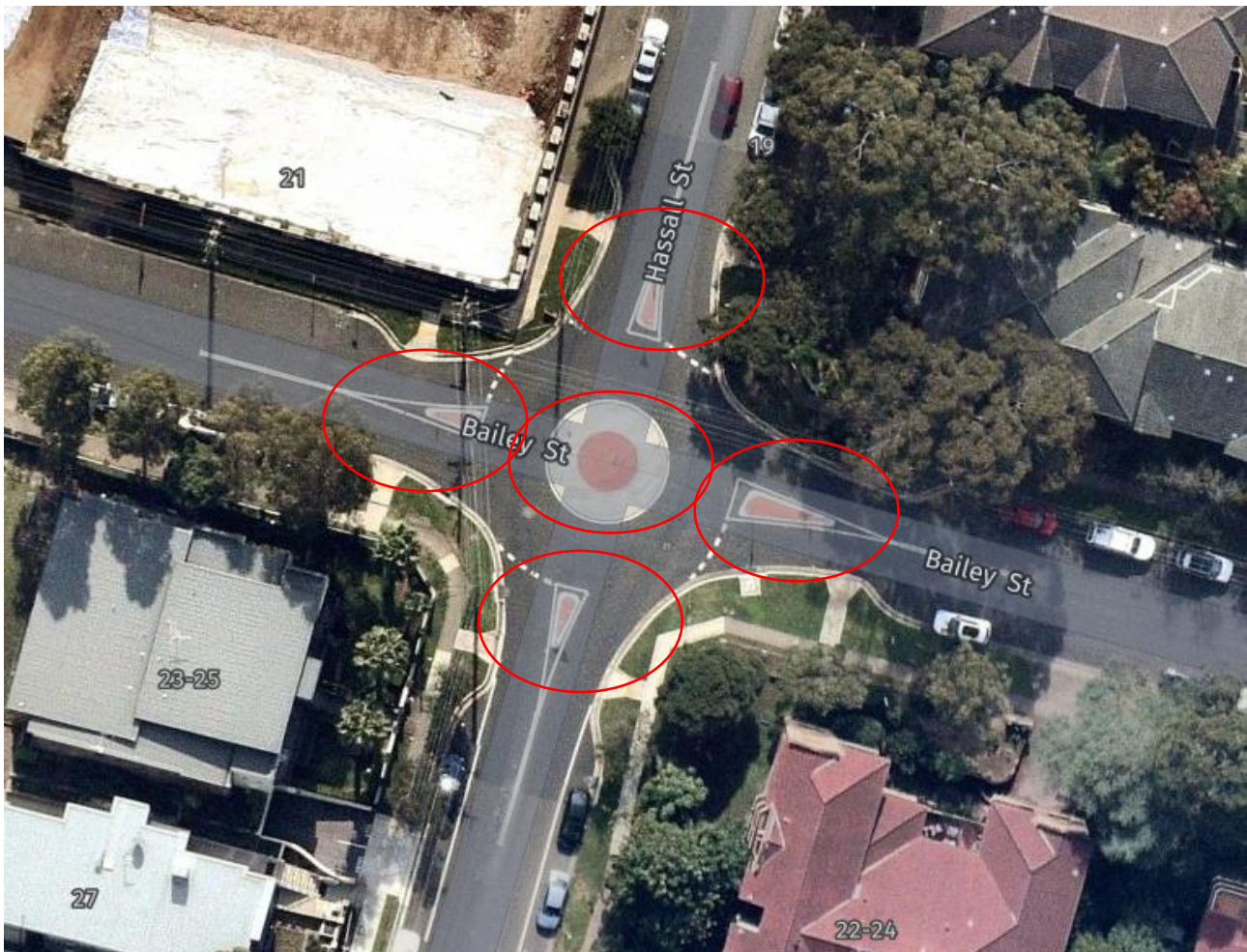
Figure 4-1: Roundabout and splitter islands to be removed
