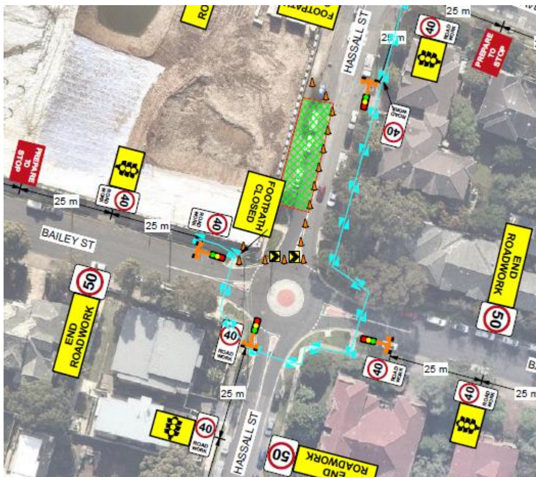
Figure 4-5: Portable traffic signal arrangements for the driveway construction
