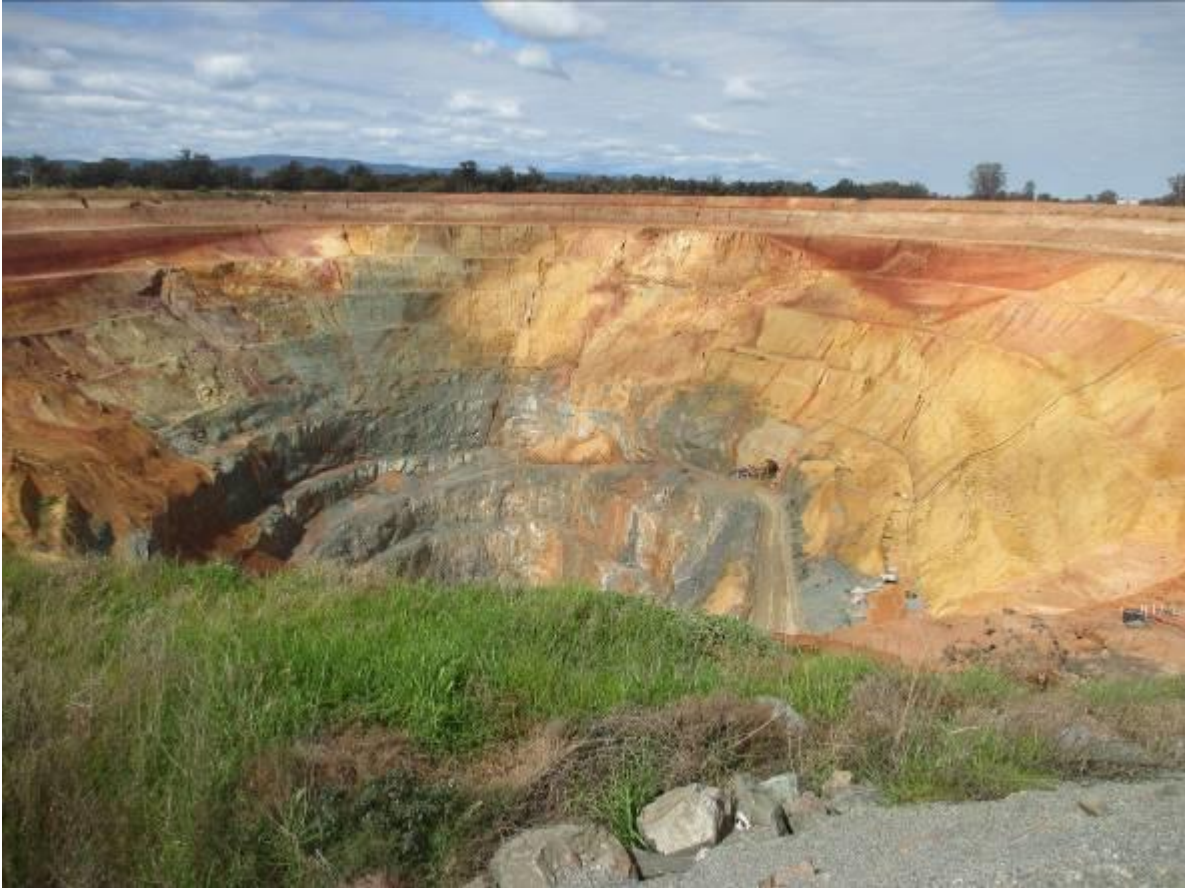
Figure 2: Wyoming 1 Open Cut looking east. Underground access portal can be viewed in the middle to the right of the image. Structure and fabric of the walls can be observed with mass failures on the opposite side.
