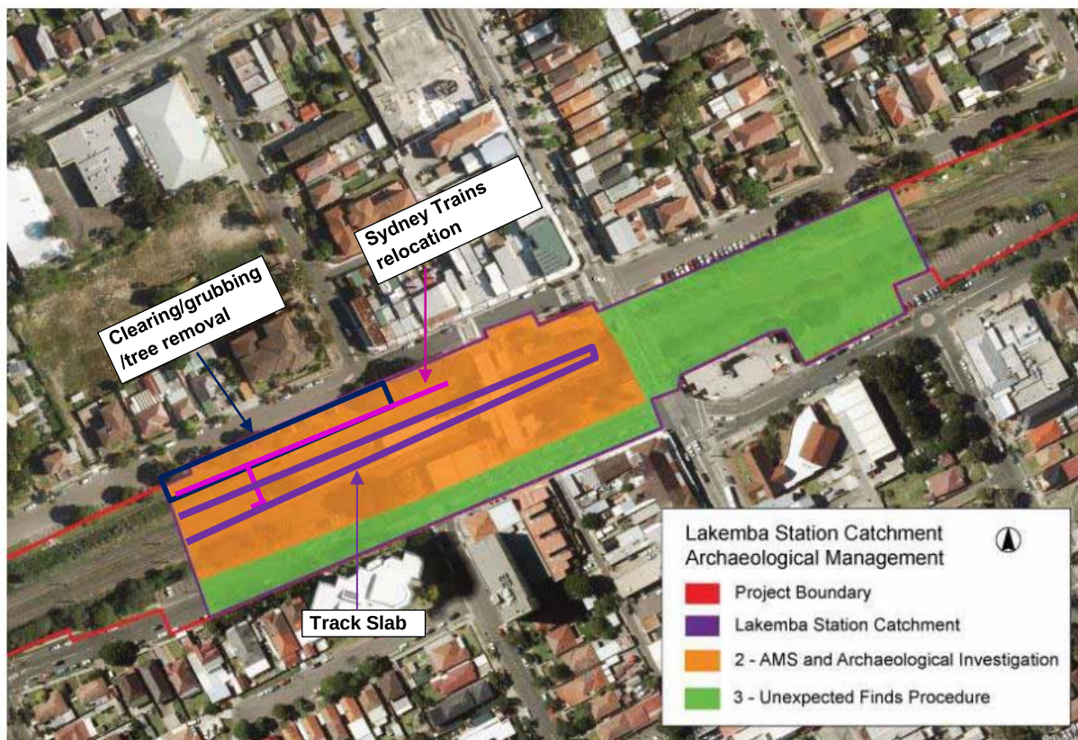
Figure 29: Primary proposed excavation works within Lakemba Station
