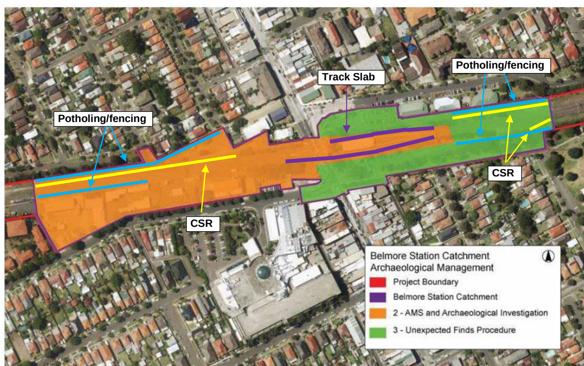
Figure 28: Primary proposed excavation works within Belmore Station
