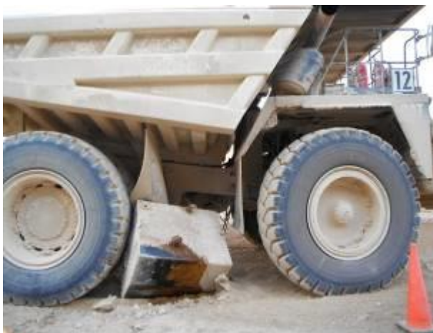
Dropped Fuel Tank. 777 Haul Truck
