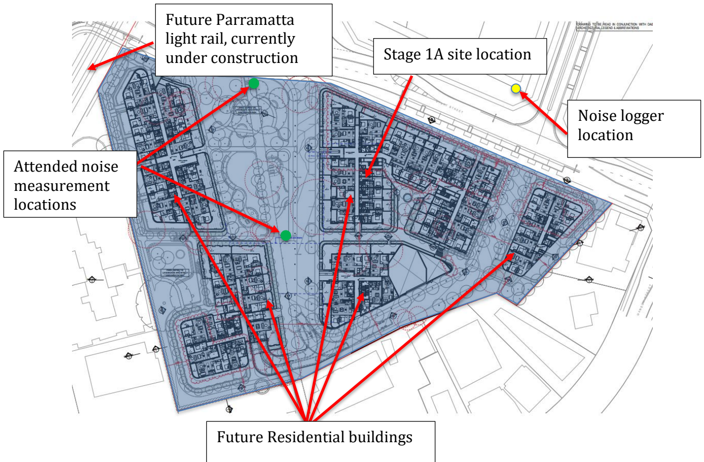
Figure 1 – Telopa Estate Stage 1A development site location
