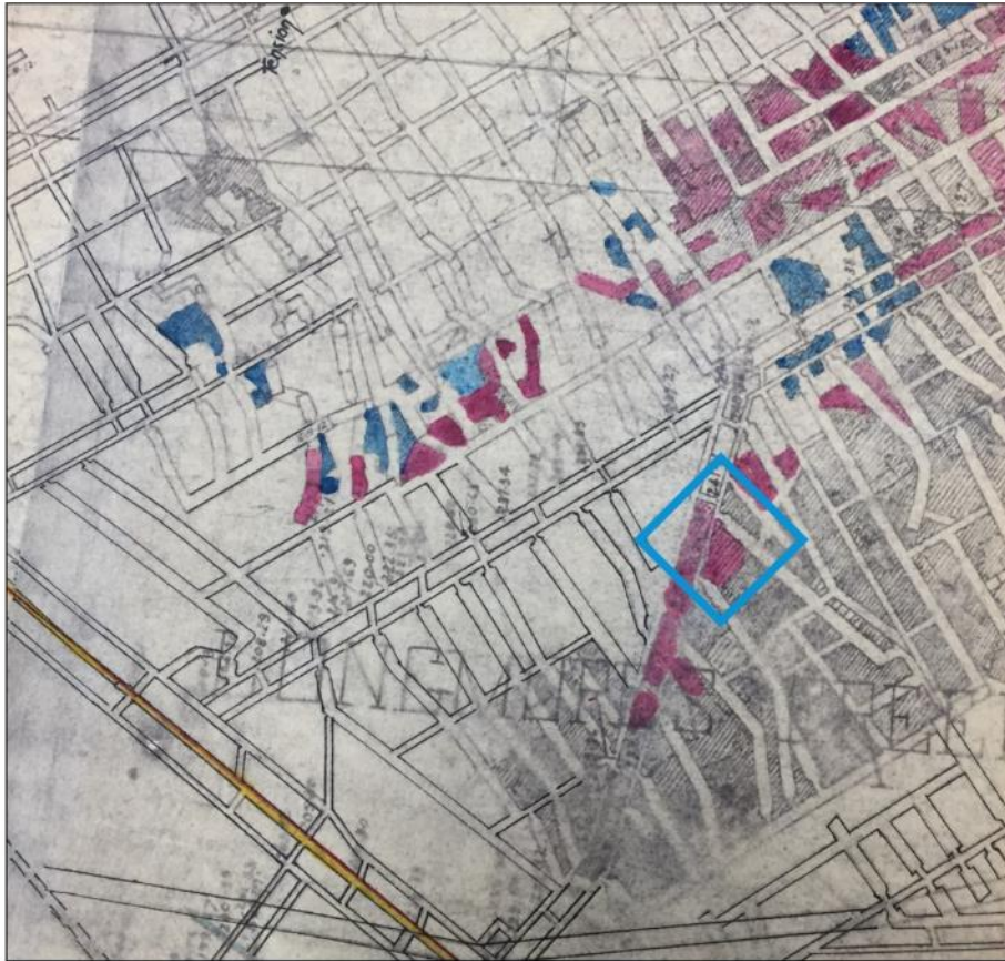
a) Position of Borehole RV16 relative to Bulli Seam workings on plan from 1916.
