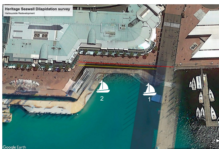
Figure 3: Location of dive survey for heritage stone seawall. Red line is extant stone wall within the study area and the yellow line is the length of stone wall the diver surveyed. Boat icons indicate approximate locations of dive vessel.
