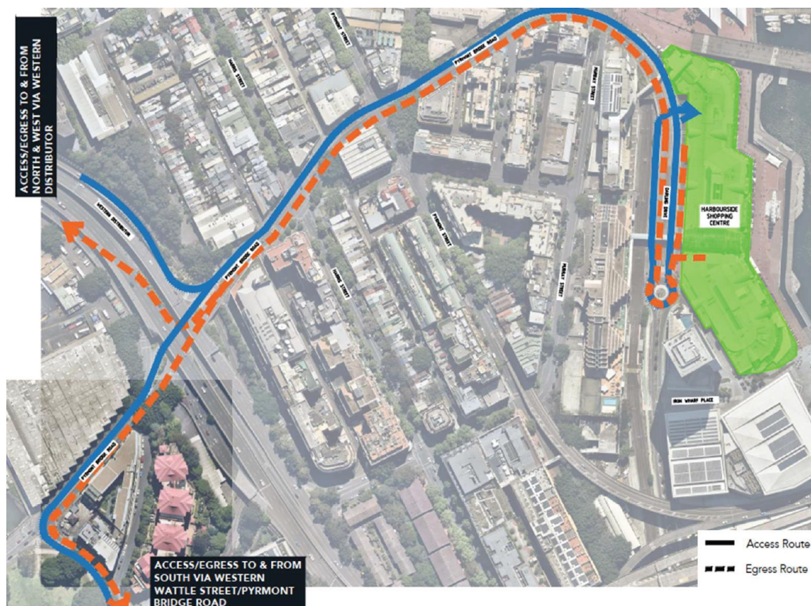
Figure 14 Construction vehicle access and egress routes
