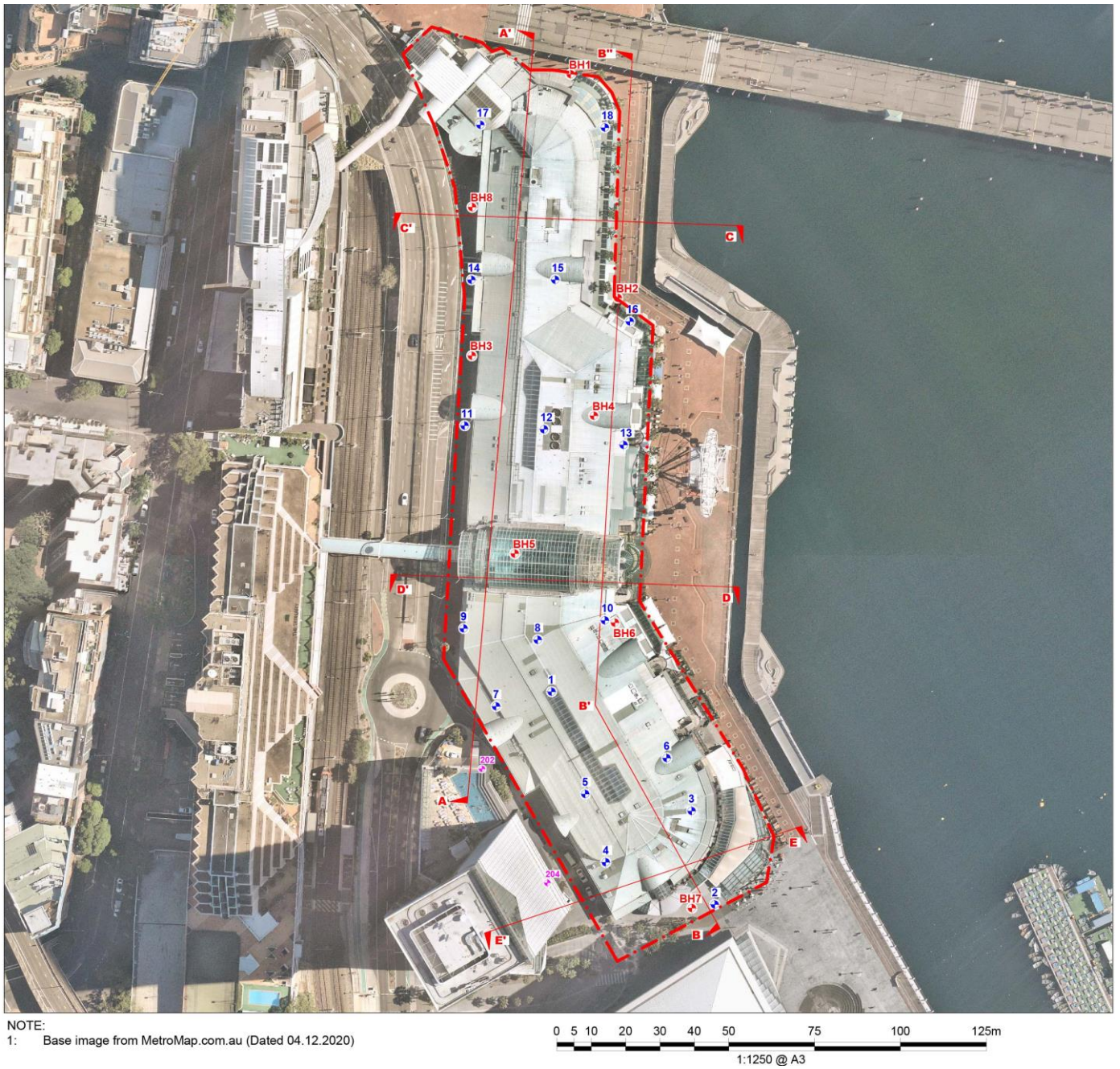
Figure 3-4 Geotechnical investigations Harbourside. The red borehole numbers correspond to the current work, the pink to the 2013 and the blue to the 1985 boreholes respectively. (Source: Douglas Partners)
