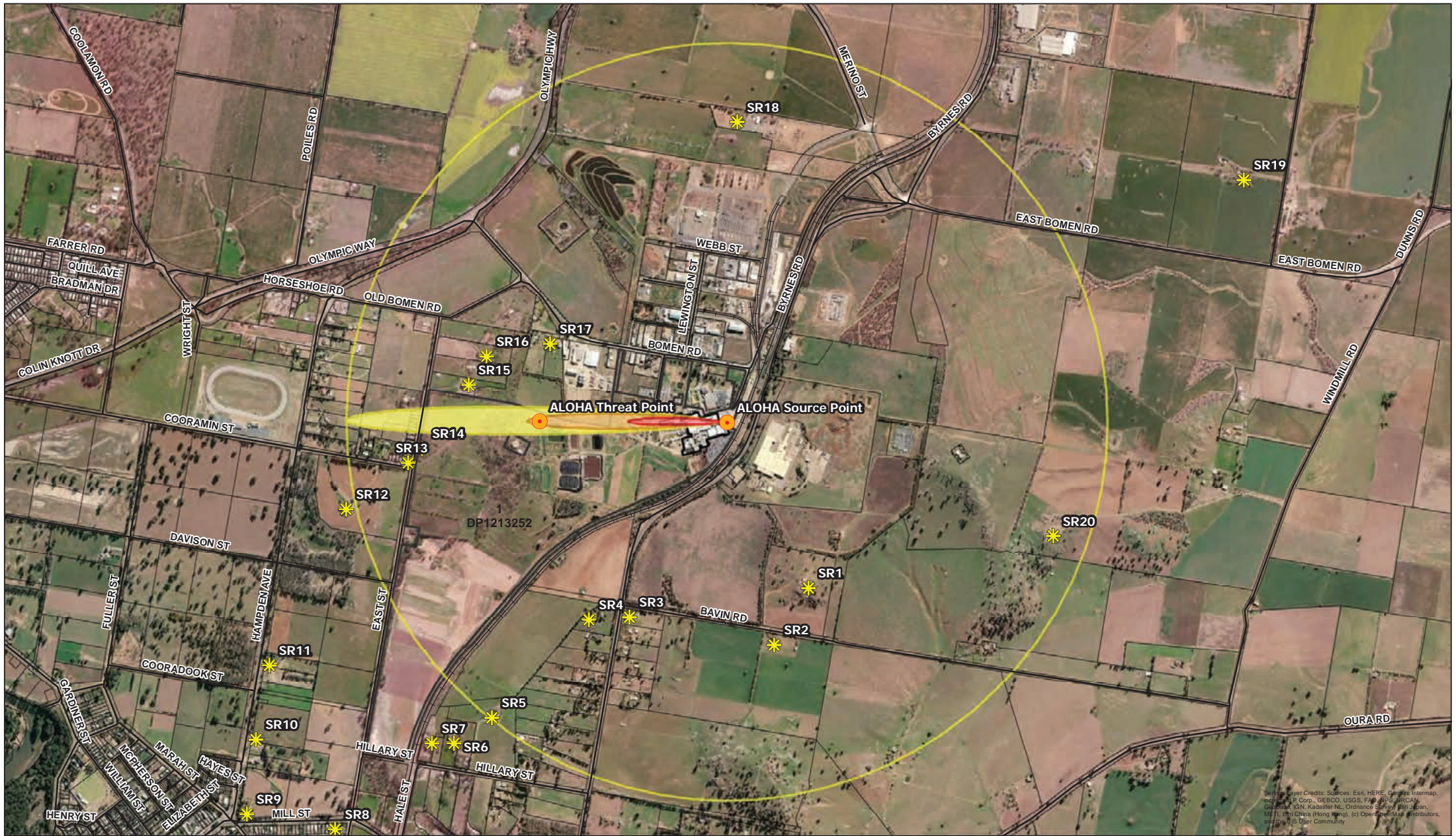
Figure 15: Hazard Modelling Scenario 2 - Worse Case Conditions; Toxic and Flammable Area of Vapour Cloud
