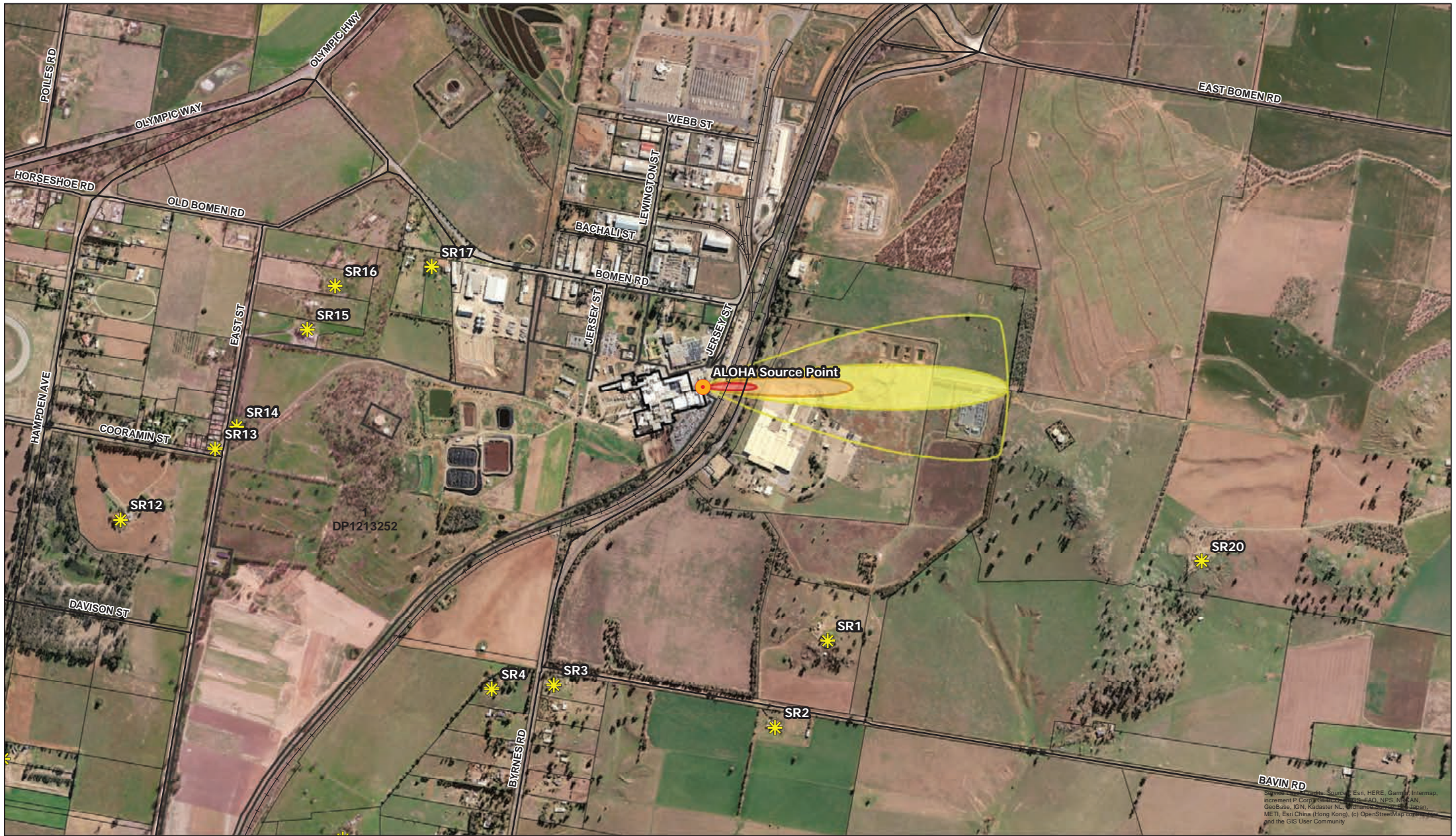
Figure 16: Hazard Modelling Scenario 2 - Normal Conditions; Toxic Area of Vapour Cloud
