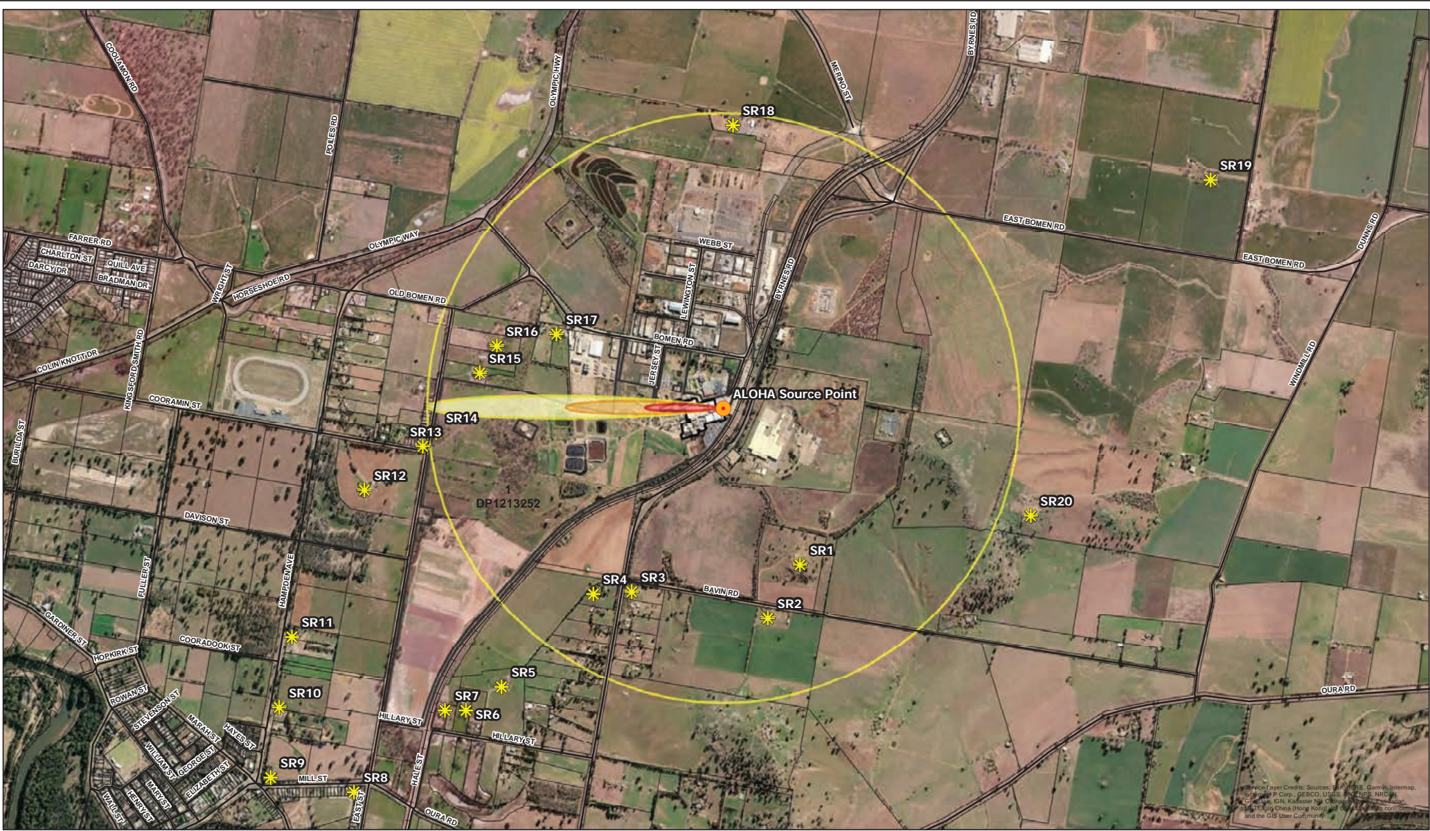
Figure 11: Hazard Modelling Scenario 1 - Worse Case Conditions; Toxic Area of Vapour Cloud
