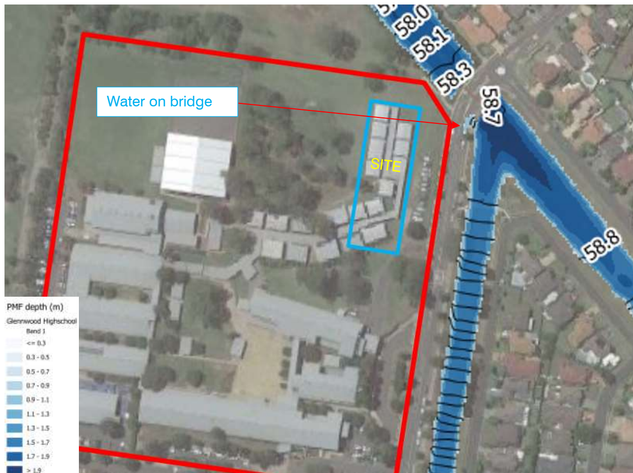
Figure 5: 1% AEP event water accumulating on the Glenwood Park Drive bridge
