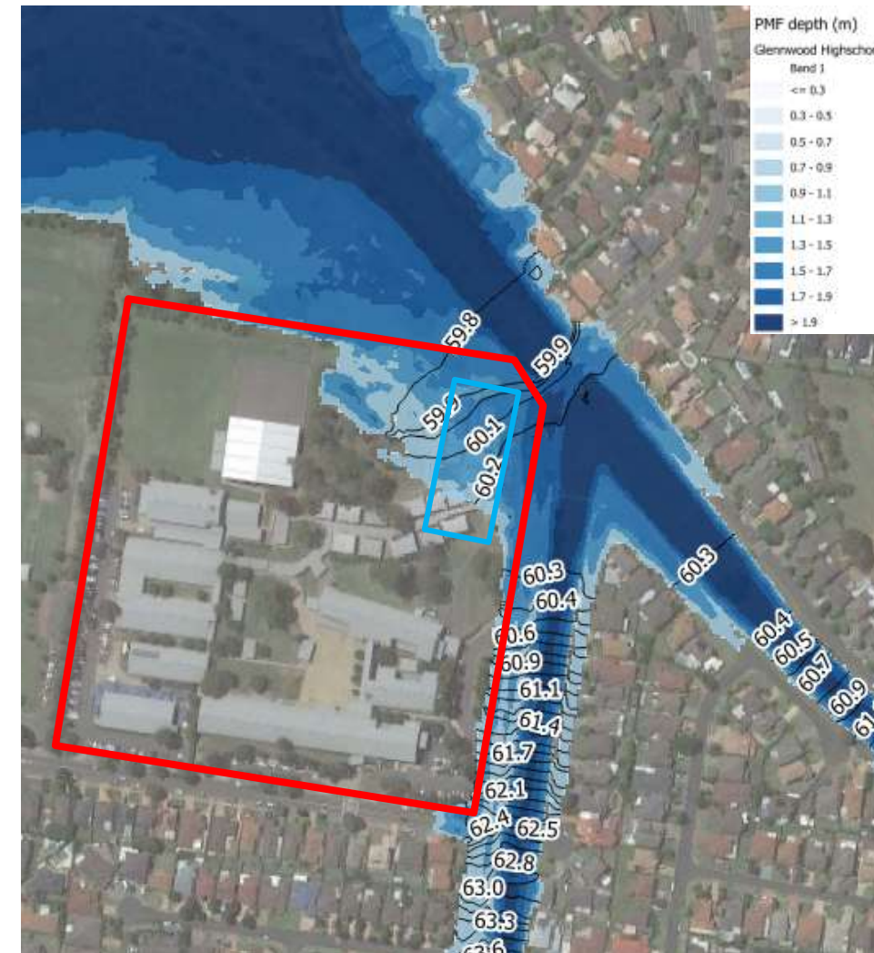
Figure 6: PMF event water accumulating on the Glenwood Park Drive bridge as riverine flooding
