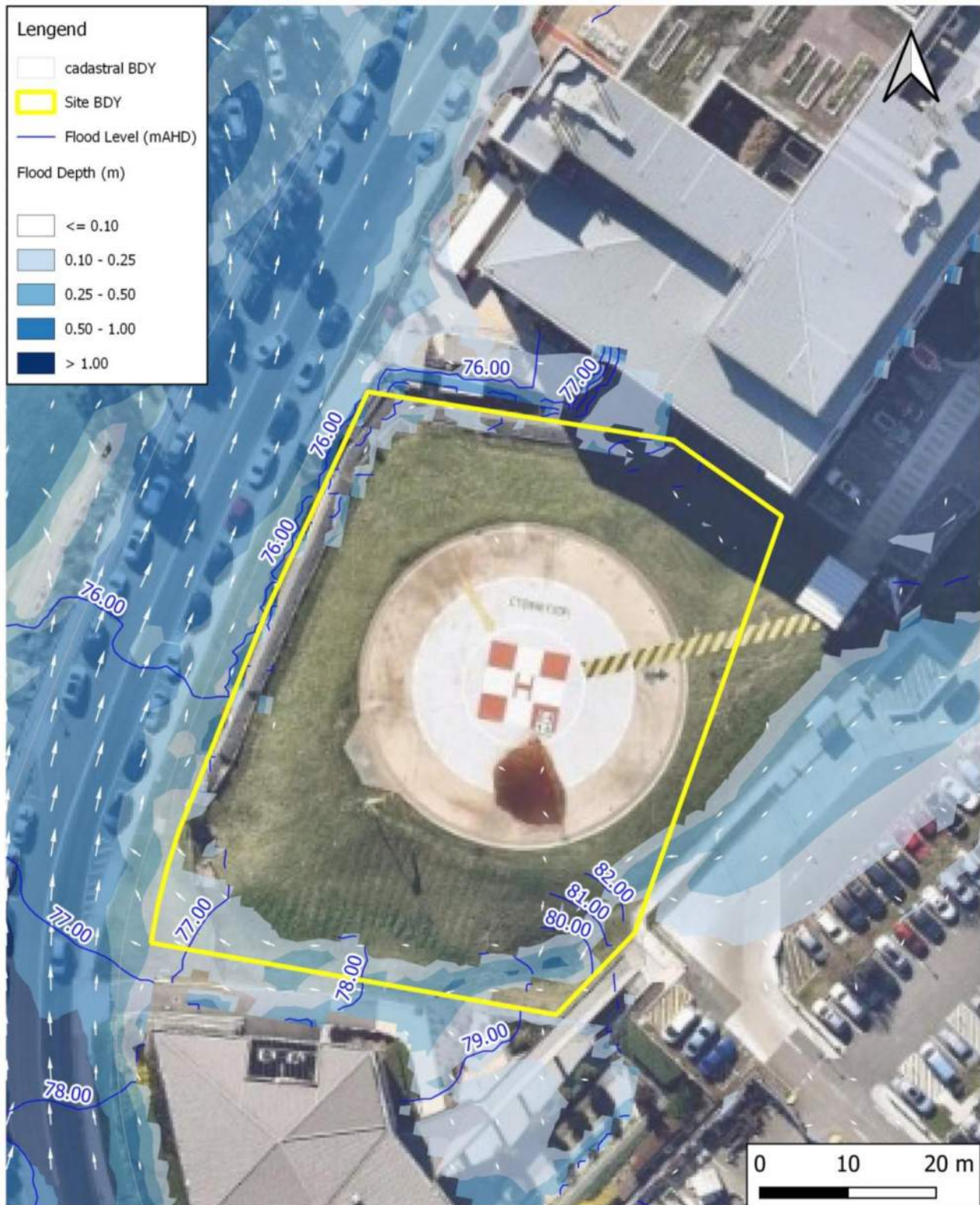
Figure 11 - Flood Levels & Depths (PMF) – Existing Conditions
