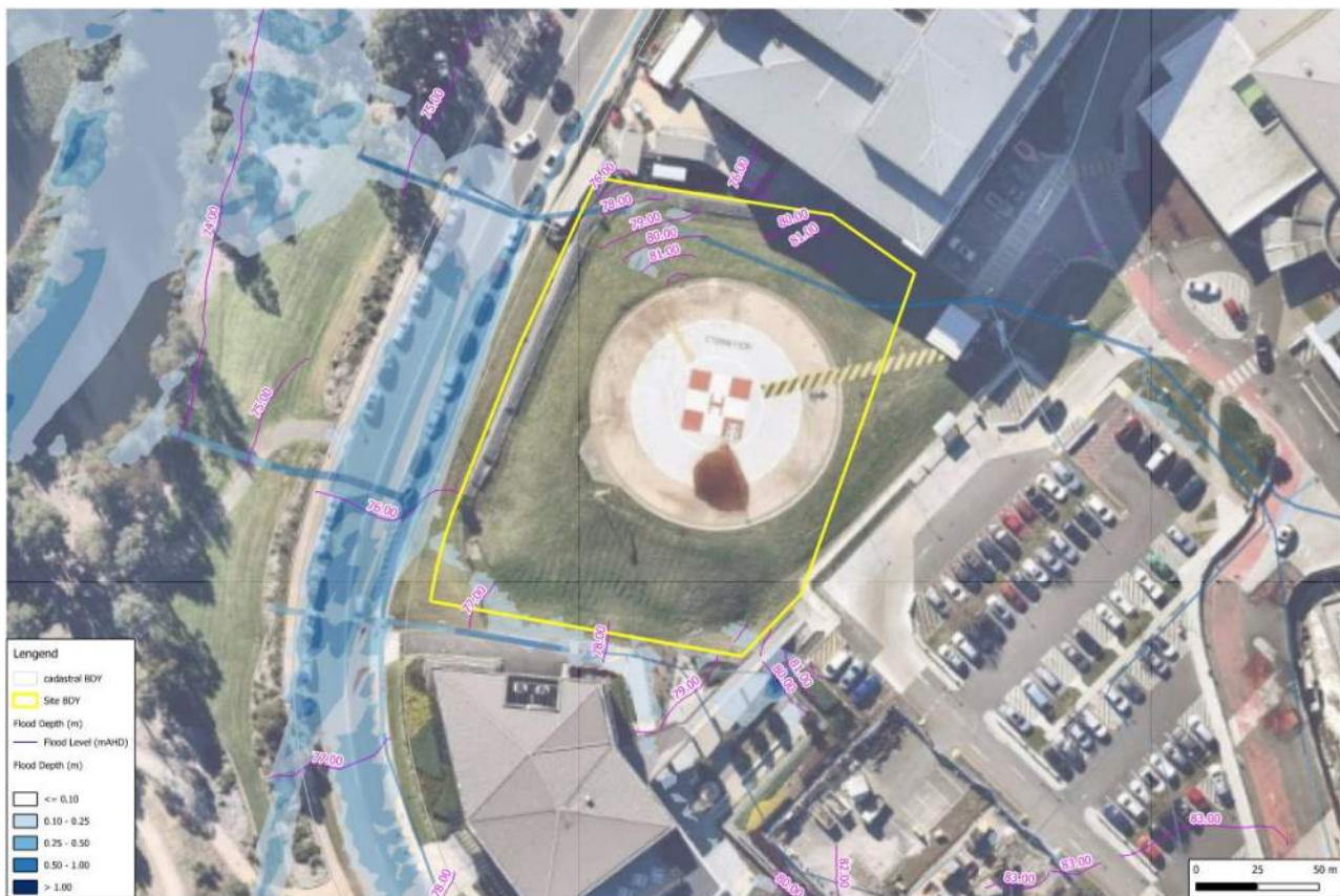
Figure 5 - Received flood Results (CSS) - 1% AEP Flood Event
