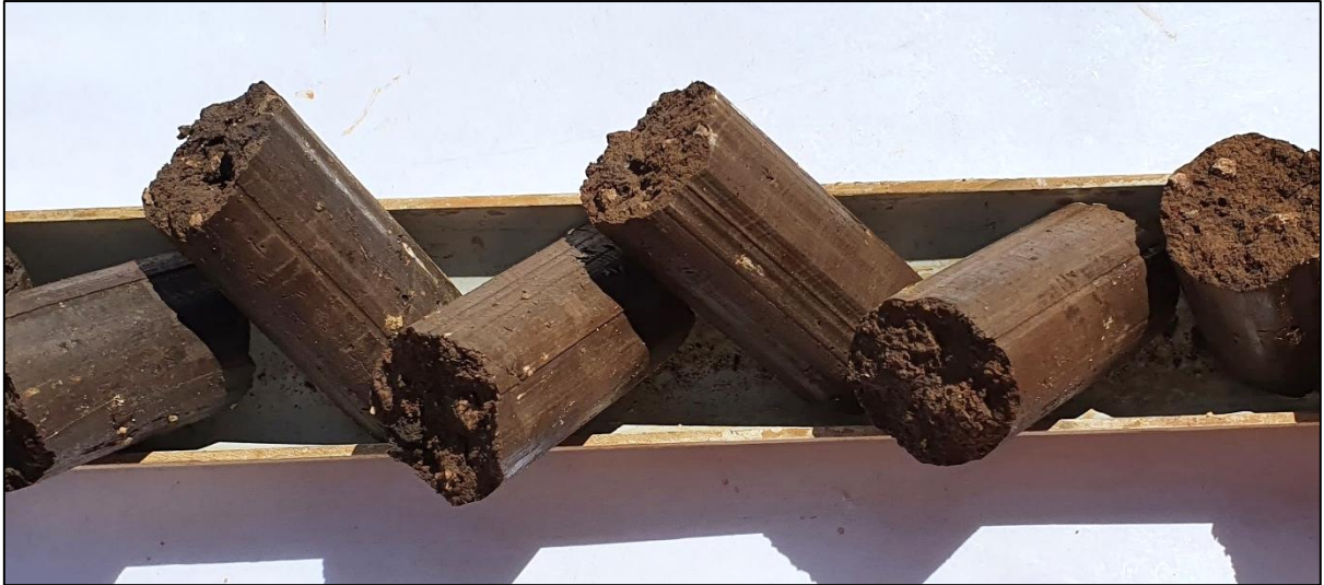
Figure 3: Bore 101, SPT 1.0 – 1.45 m, very stiff to hard silty clay.
