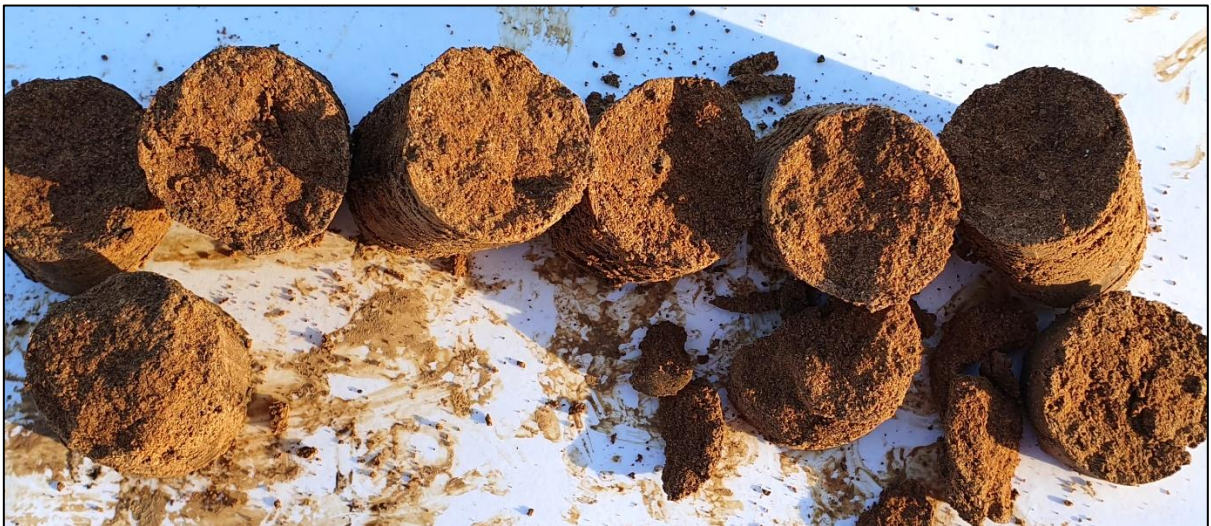
Figure 4: Bore 104, SPT 2.5 – 2.95 m, dense to very dense silty sand with clay.
