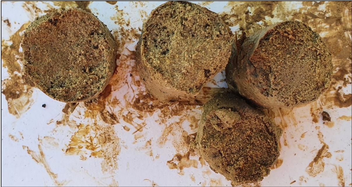
Figure 5: Bore 105, SPT 7.0 – 7.30 m, very dense clayey sand.
