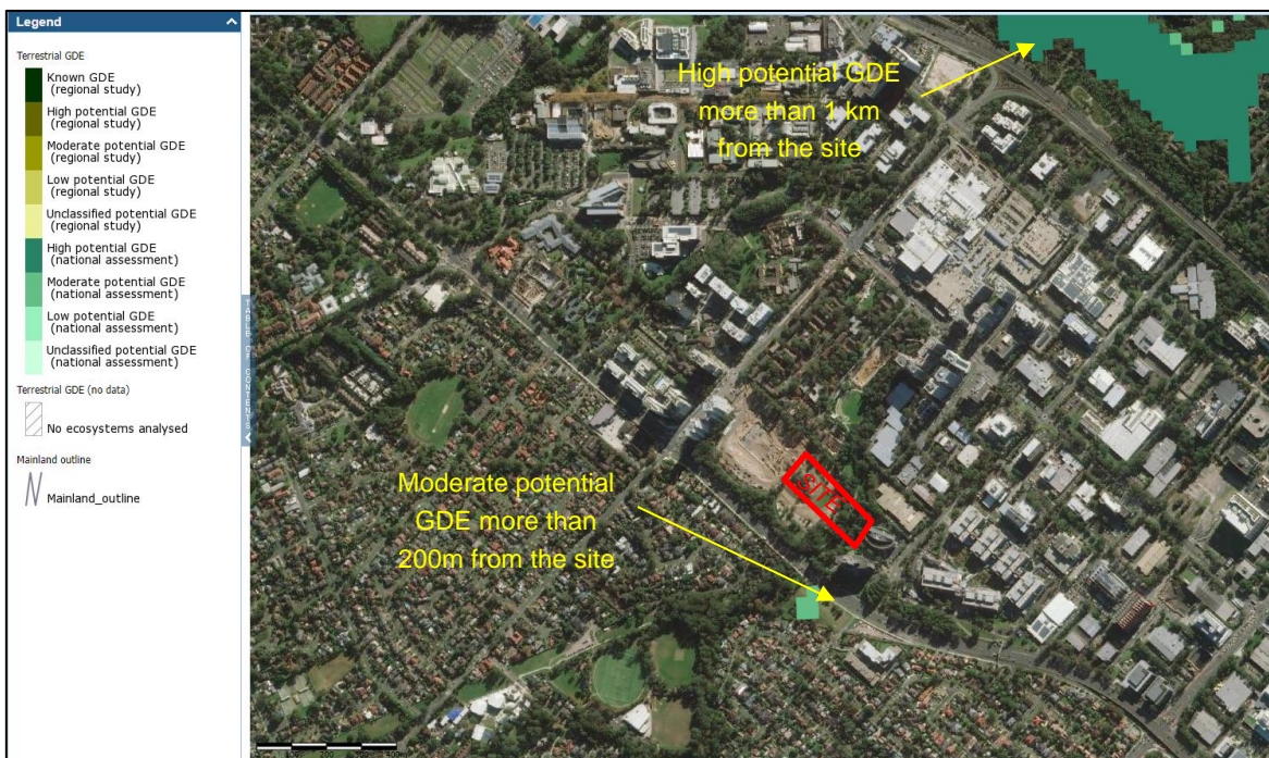
Figure 5: Map of Groundwater Dependent Ecosystems (GDEs) Near the Site (Bureau of Meteorology (BoM): GDE Atlas online, viewed 28 April 2022.)
