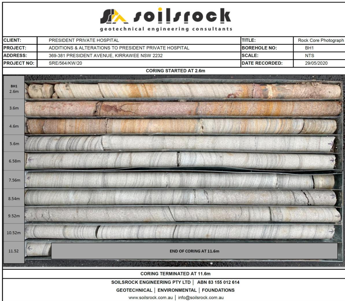
Figure 6-6 Geotechnical Bore Log BH1 - Rock Core Photograph. Soilsrock Engineering Pty Ltd, 2020.
