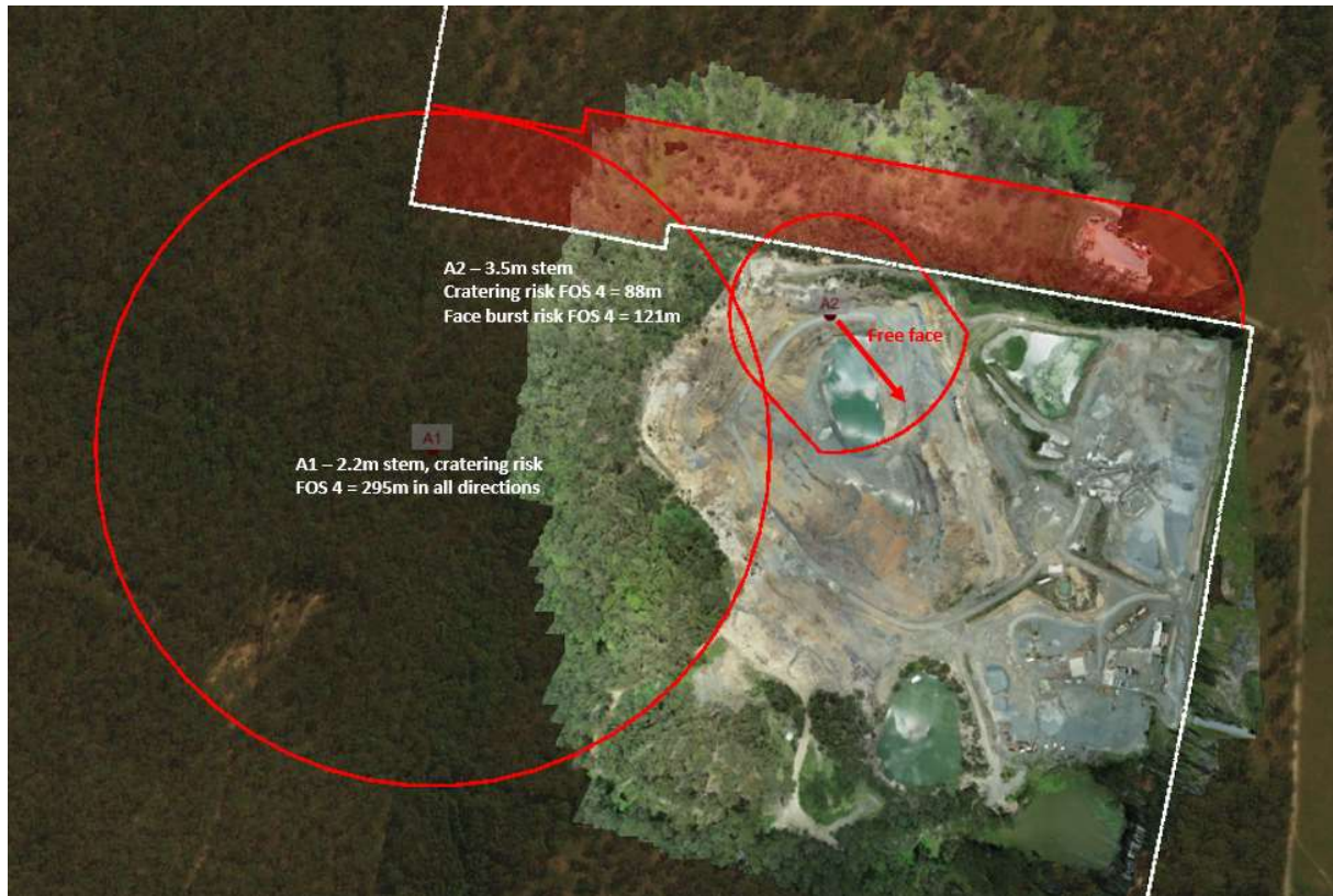
Figure 13 - Exclusion zone distance illustration for recommended controls (89mm blastholes)
