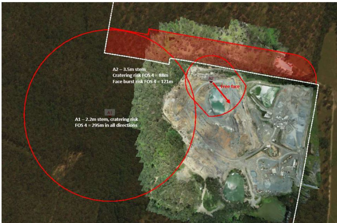
Figure 3: Recommended exclusion zone required for two different drill and blast design parameters (with 89mm blastholes). The two scenarios indicate that increase stemming heights of blastholes reduces the required size of the blasting exclusion zone (Figure 13, Buffer Zone Assessment Report, Orica 2022).
