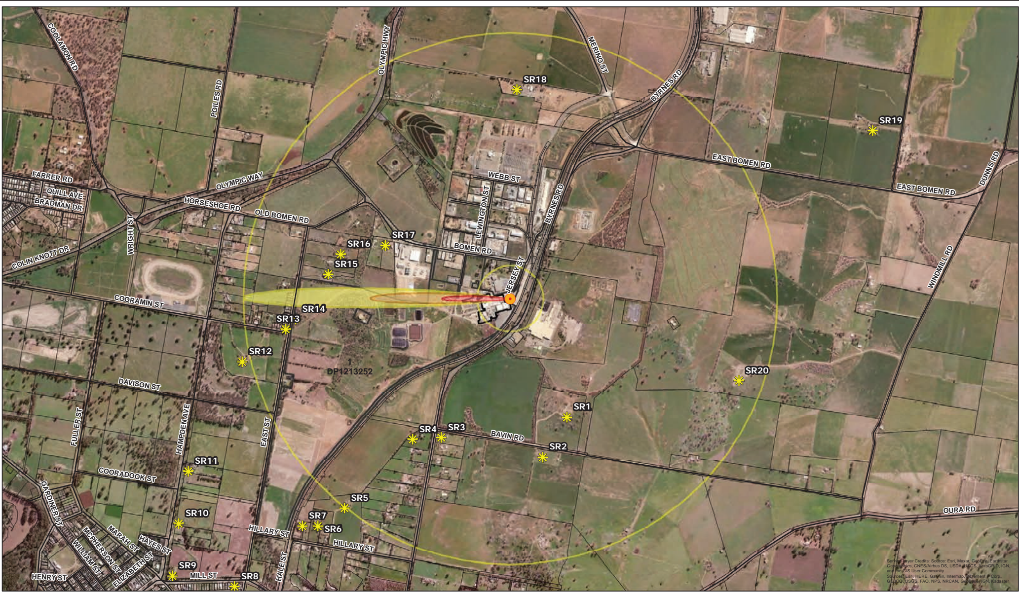
Figure 15: Hazard Modelling Scenario 2 - Worst Case Conditions; Toxic and Flammable Area of Vapour Cloud
