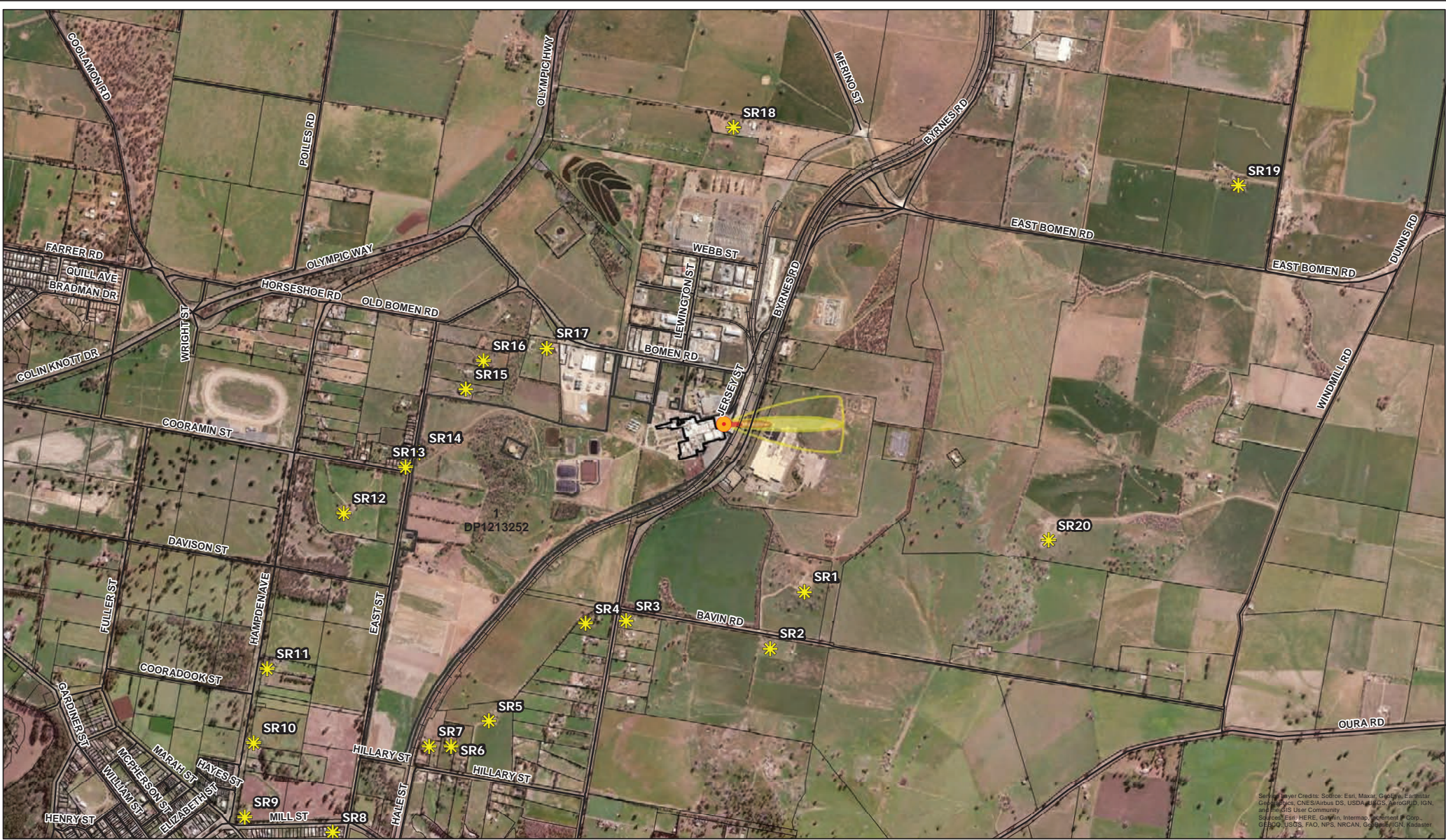
Figure 20: Hazard Modelling Scenario 3 - Normal Conditions; Toxic Area of Vapour Cloud
