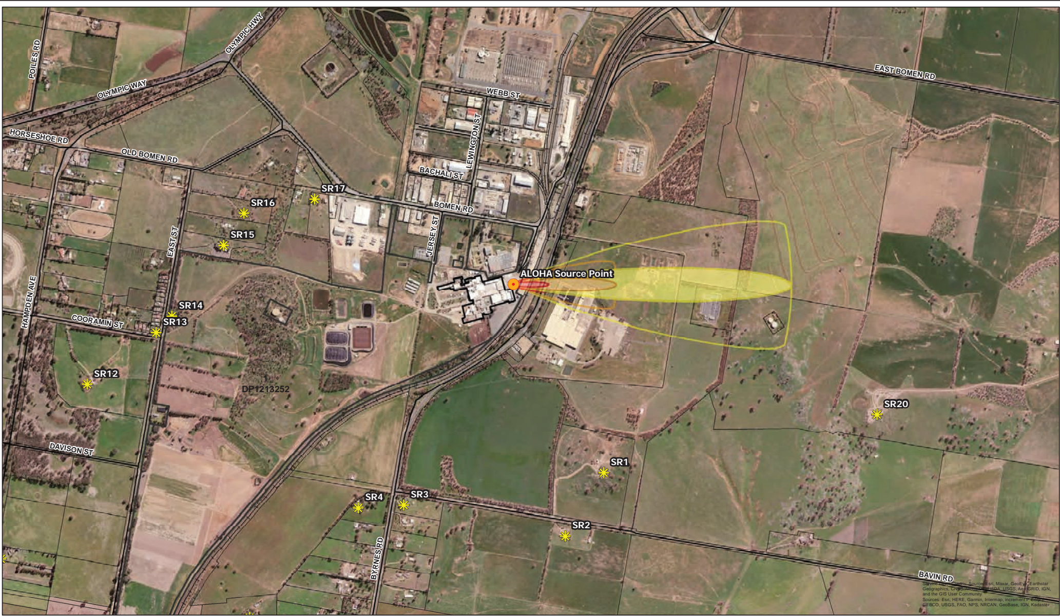
Figure 12: Hazard Modelling Scenario 1 - Normal Conditions; Toxic Area of Vapour Cloud
