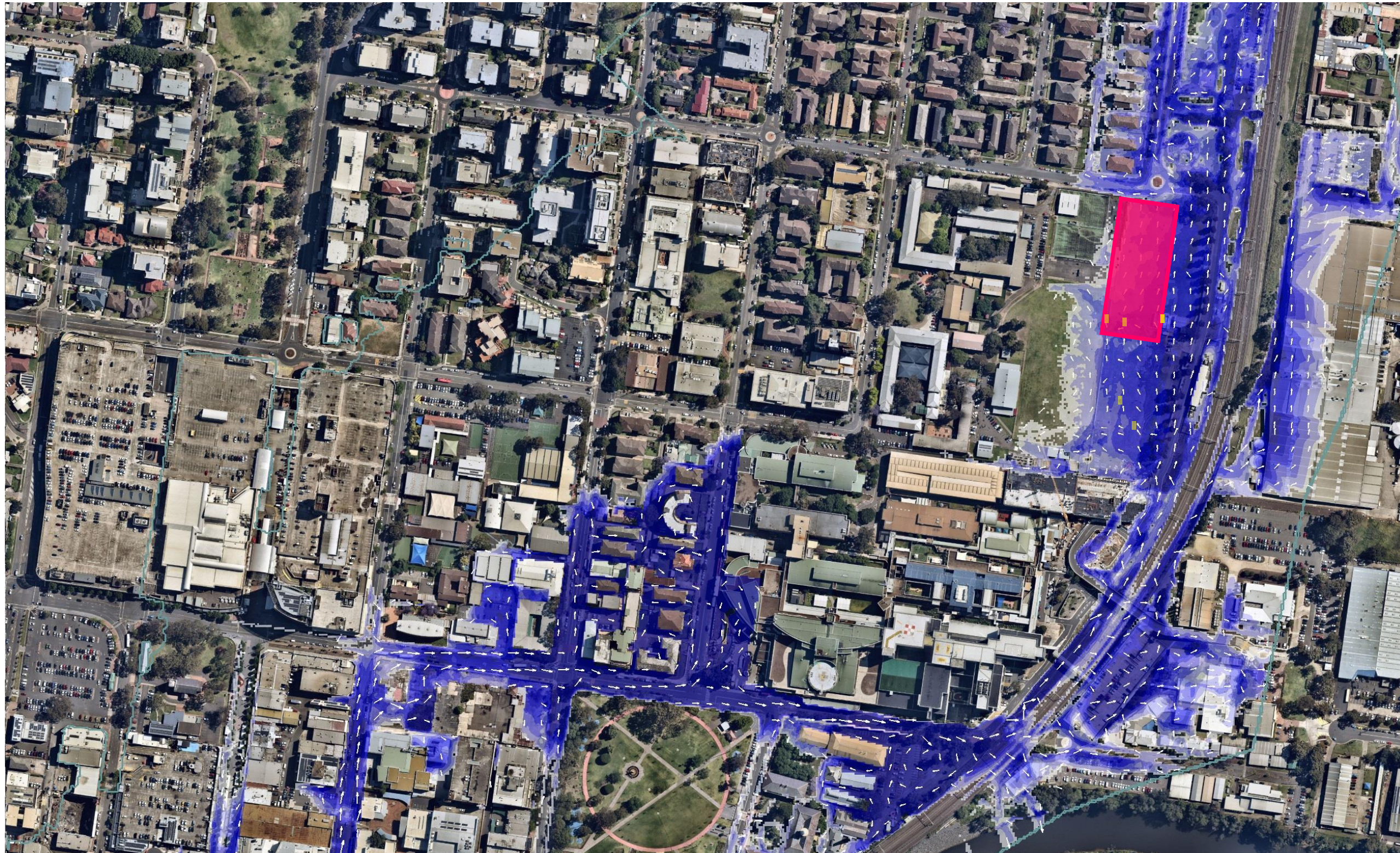
Figure 4: PMF Flood Extent for Mainstream and Overland Flooding with NLPS school location in red (Georges River Floodplain Risk Management Study & Plan, May 2004 and Liverpool City Centre Overland Flow Path Mapping, December 2016)
