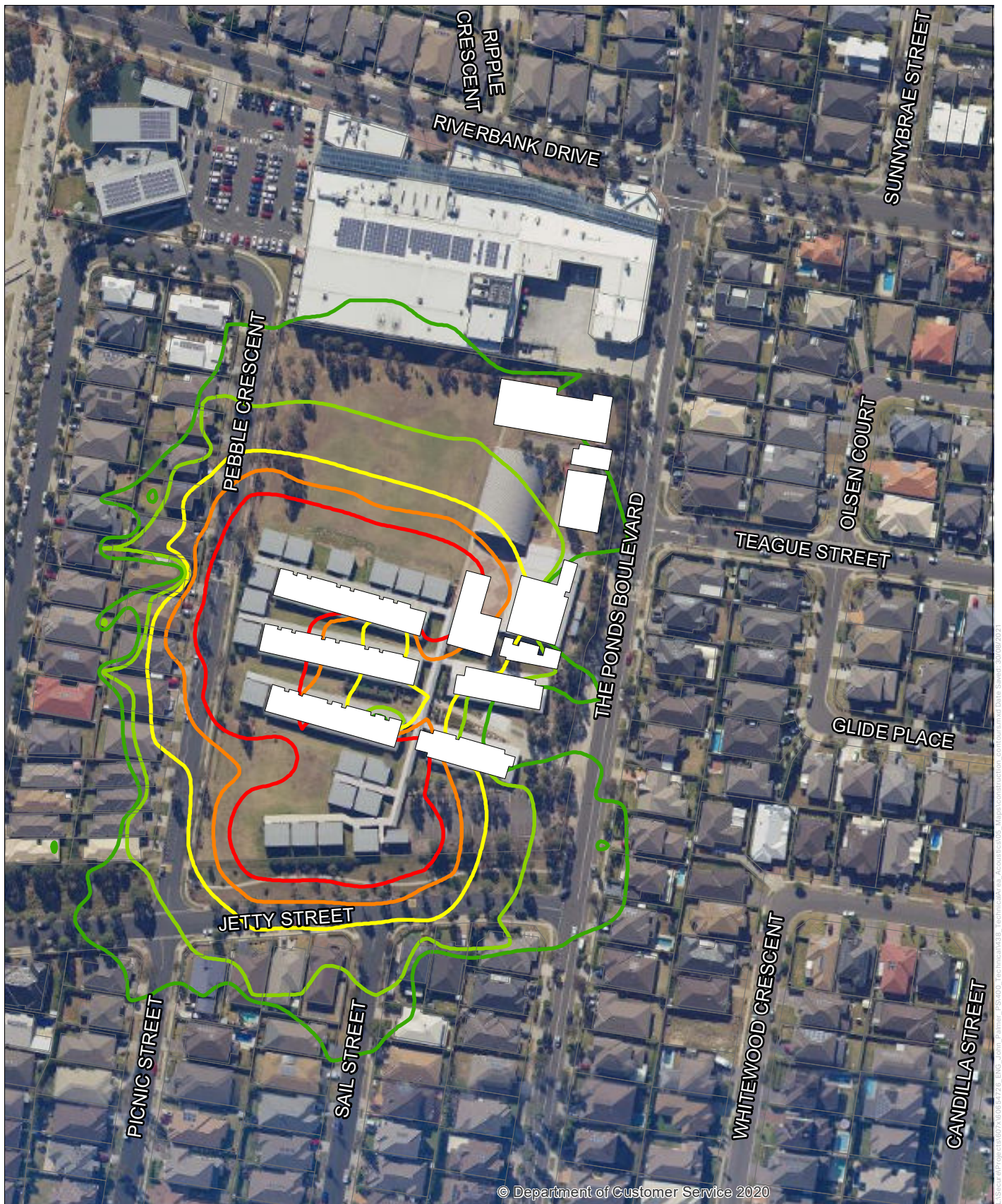
Construction Noise Contours - Demountable Removal
