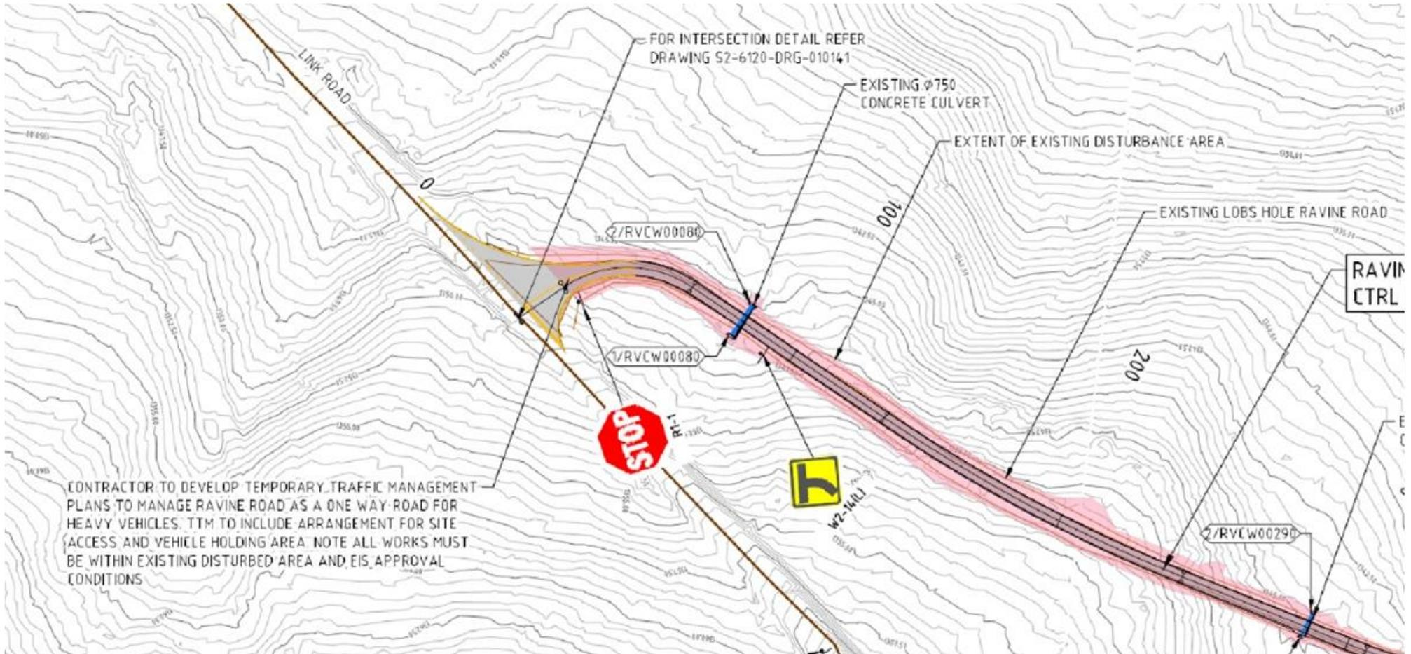
Figure 5-1: Indicative layout of lay-up area at the intersection of Link Road and Ravine Road
