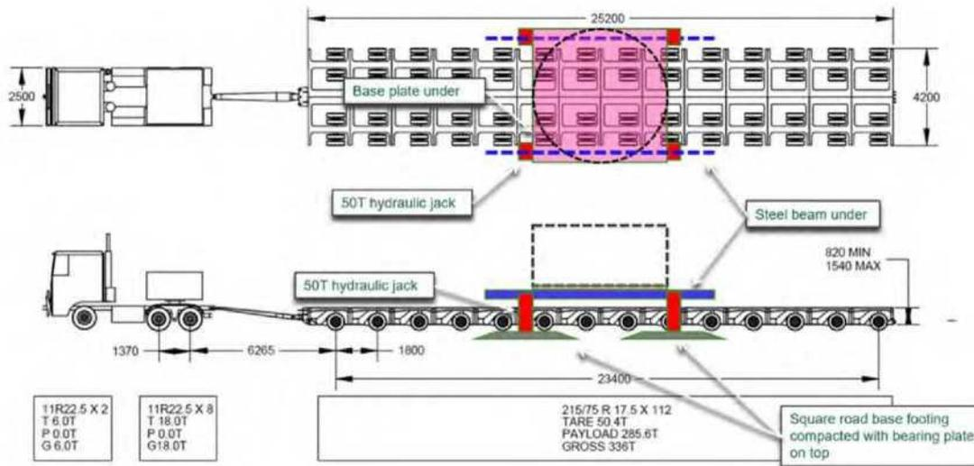
Figure 5-2: Typical OSOM configuration
