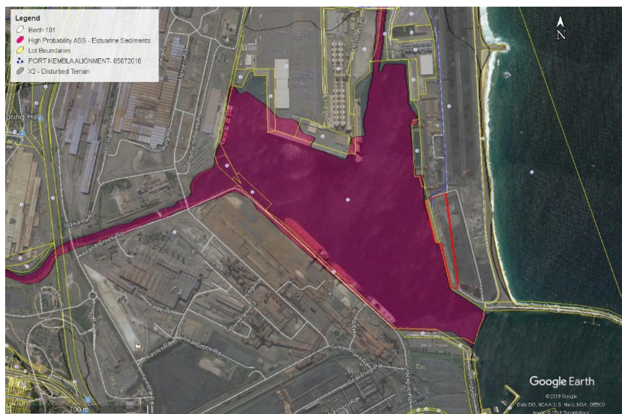
Figure 1 Wollongong ASS Risk Map showing bottom sediments (purple shading)
