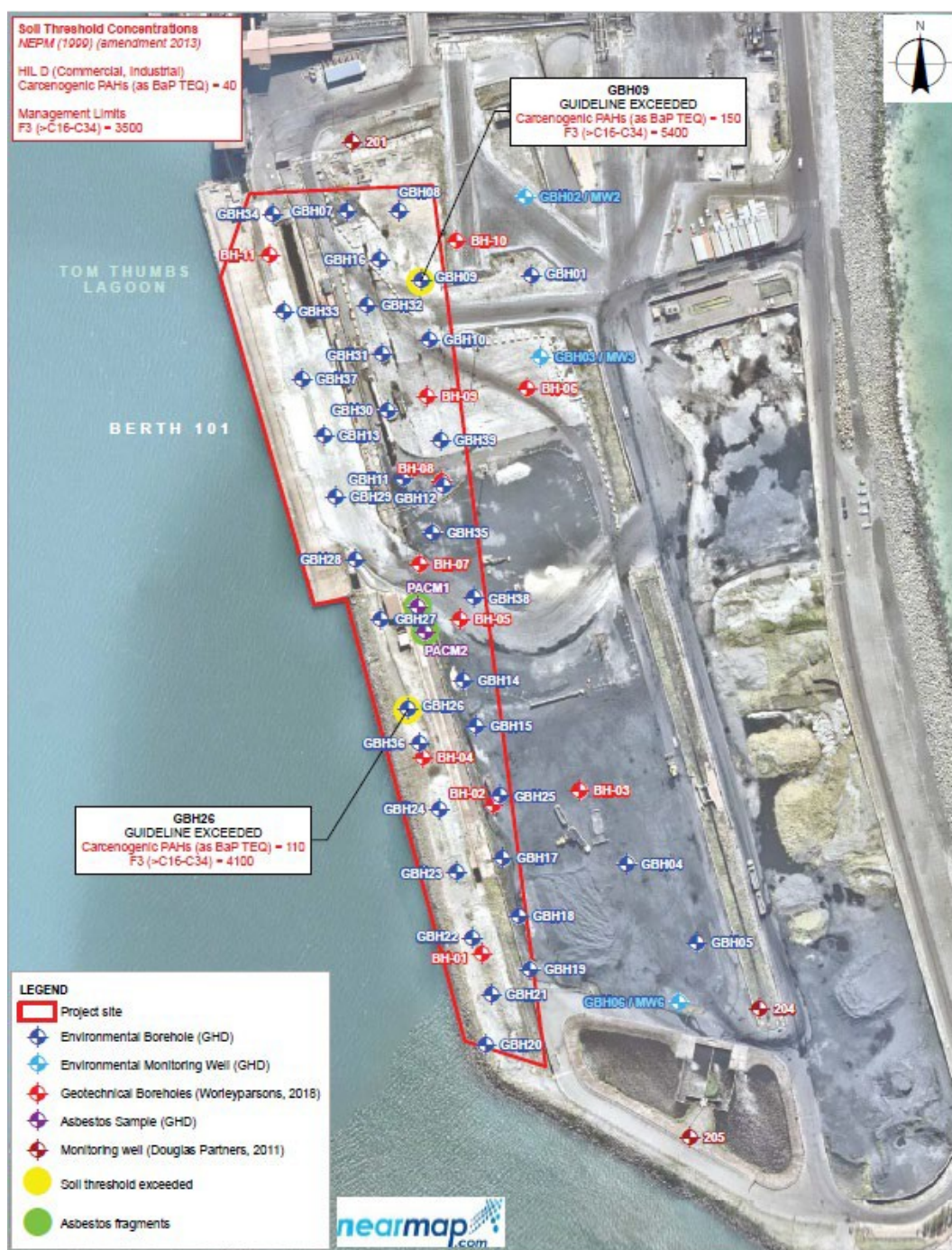
Figure 7.1 Borehole locations where ASS identified (GHD, 2018)
