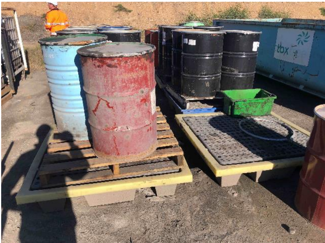
Plate 12 - Drums located on banded pallets near workshop.
