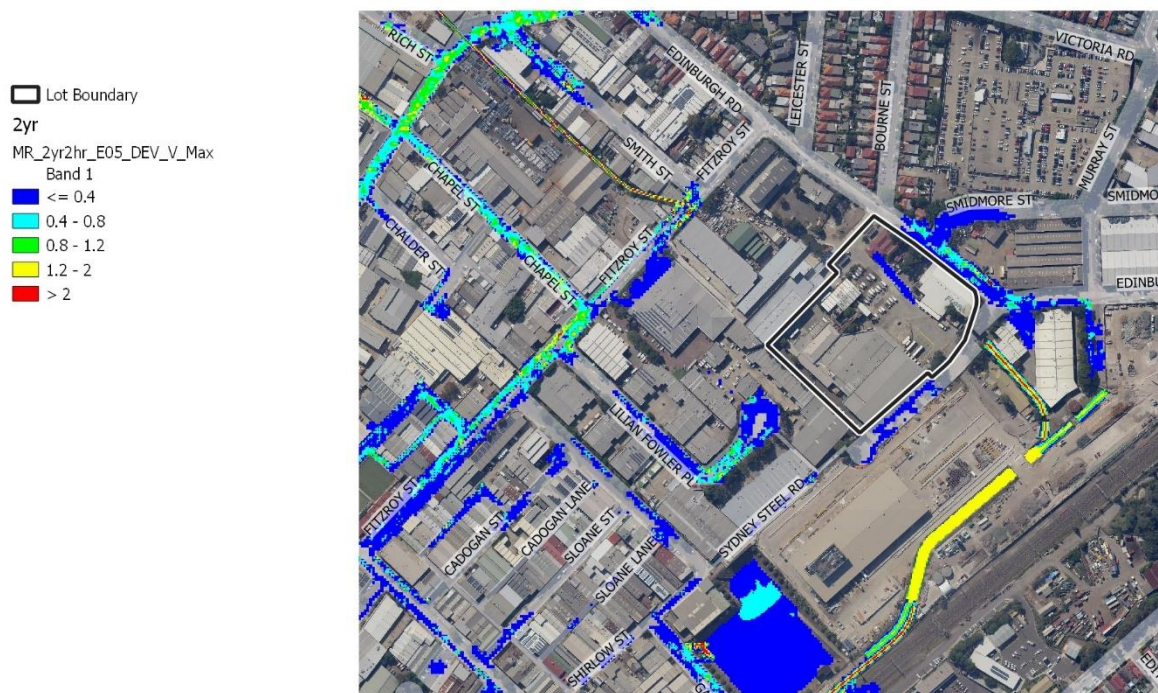
Figure 24 Post Development 50% AEP Flood Velocity (m/s)
