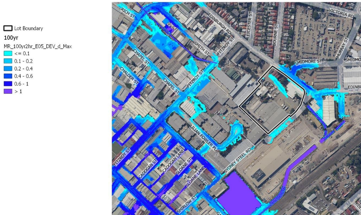
Figure 32 Post Development 1% AEP Flood Depth (m)
