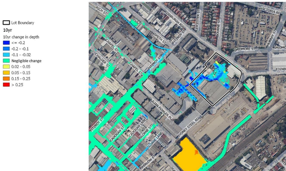
Figure 41 Post Development change in 10% AEP flood depth (m)
