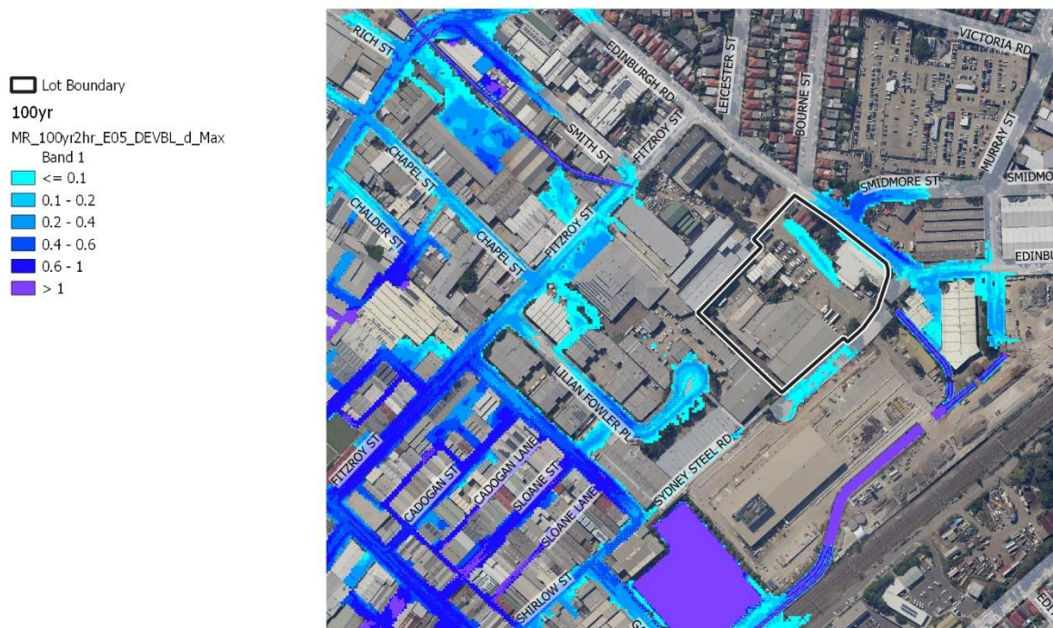
Figure 33 Post Development 1% AEP Flood Depth – Blockage scenario – Grate blocked (m)
