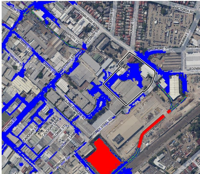
Figure 13 Pre Development 20% AEP Flood Hazard Category
