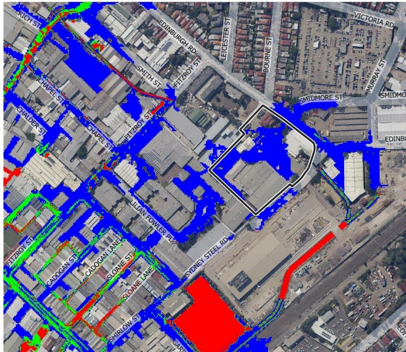
Figure 19 Pre Development 1% AEP Flood Hazard Category
