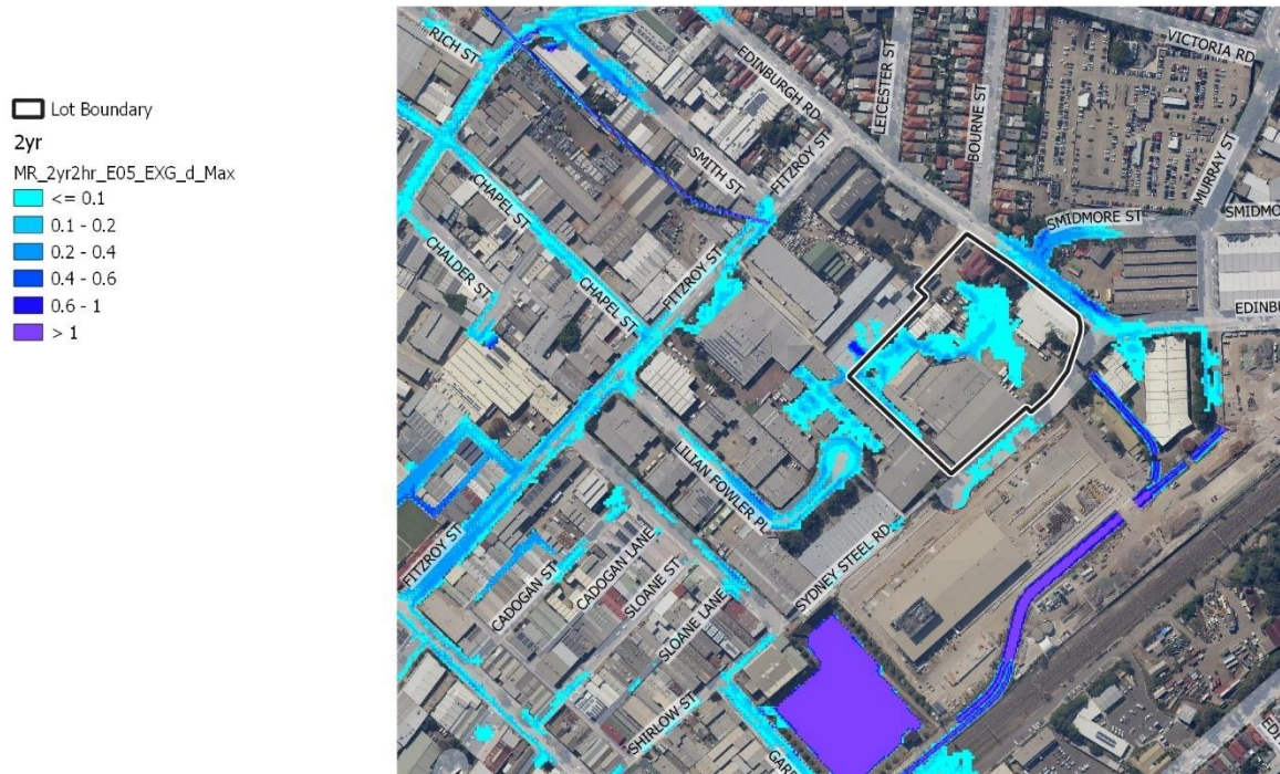
Figure 8 Pre Development 50% AEP Flood Depth (m)
