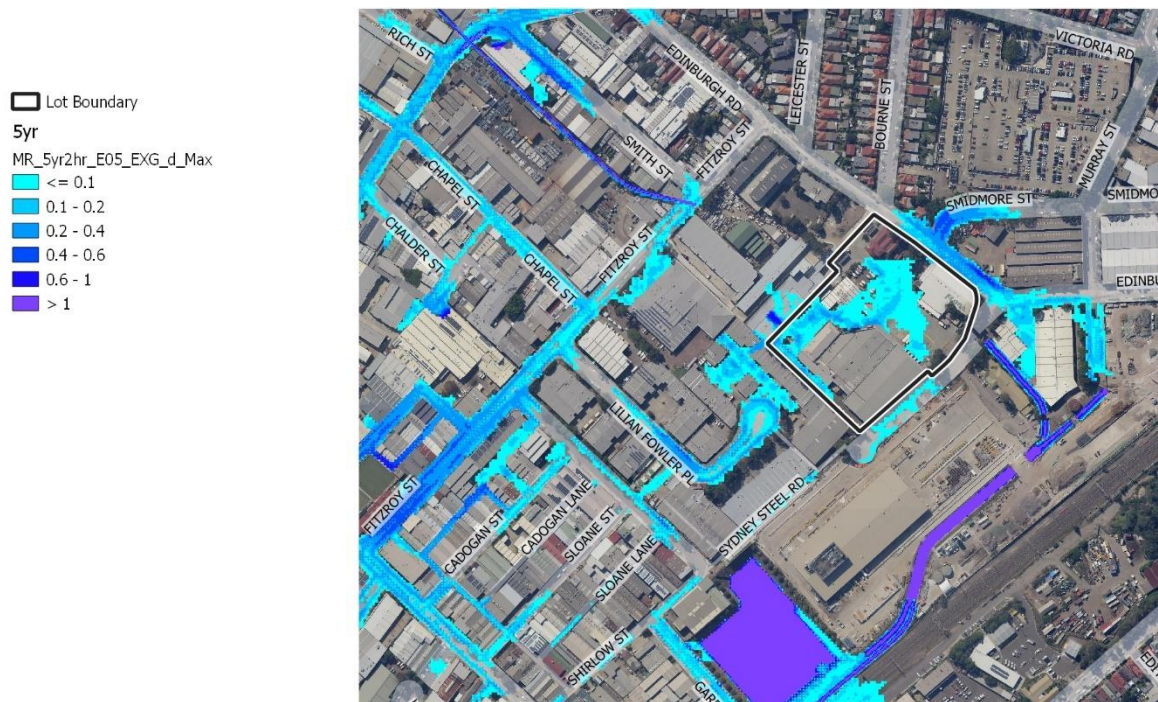
Figure 11 Pre Development 20% AEP Flood Depth (m)
