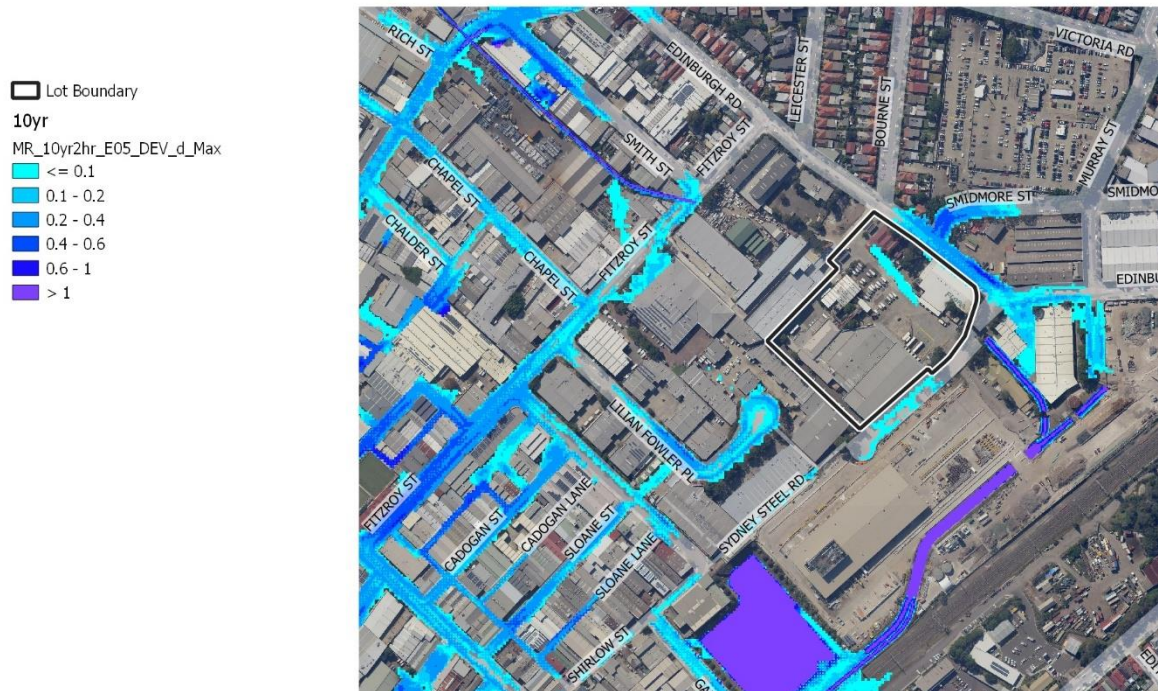
Figure 29 Post Development 10% AEP Flood Depth (m)
