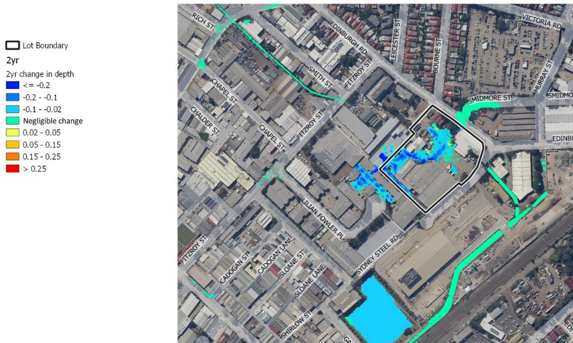
Figure 39 Post Development change in 50% AEP flood depth (m)
