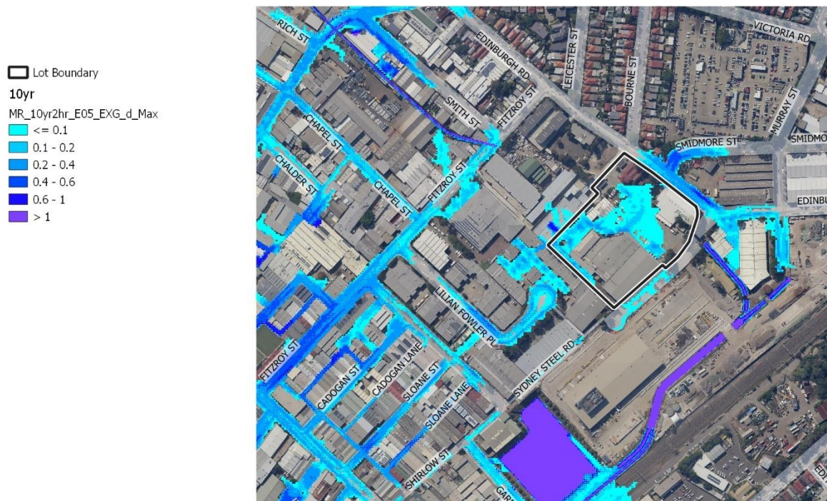
Figure 14 Pre Development 10% AEP Flood Depth (m)
