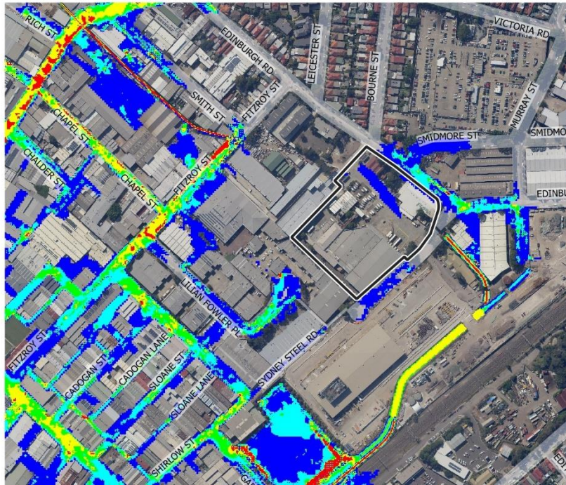
Figure 34 Post Development 1% AEP Flood Velocity (m/s)
