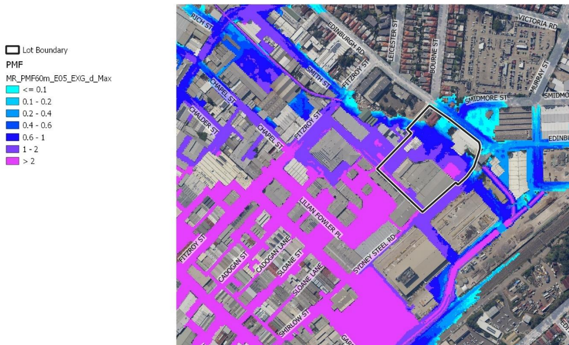
Figure 20 Pre Development PMF Flood Depth (m)
