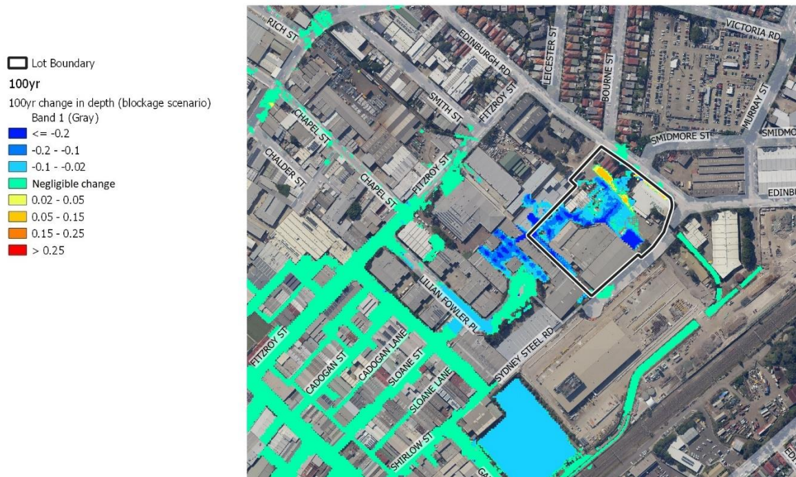
Figure 43 Post Development change in 1% AEP flood depth – Blockage Scenario – Grate Blocked (m)
