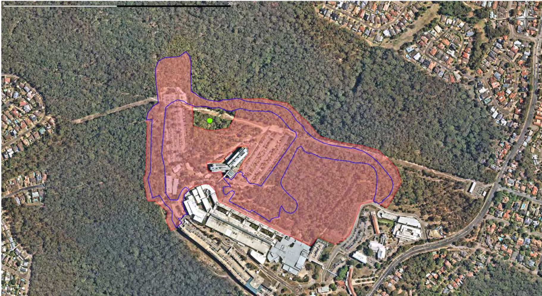
Figure 2 The current proposed works footprint is shown in blue (subject to change). Shown in red is the maximum area that may be subject to impact through changes to the proposed works footprint. The approximate location of the Yallarwah memorial is shown by the green marker, with a minimum 25 meter buffer to be established around this marker to ensure no disturbance occurs during the project.
